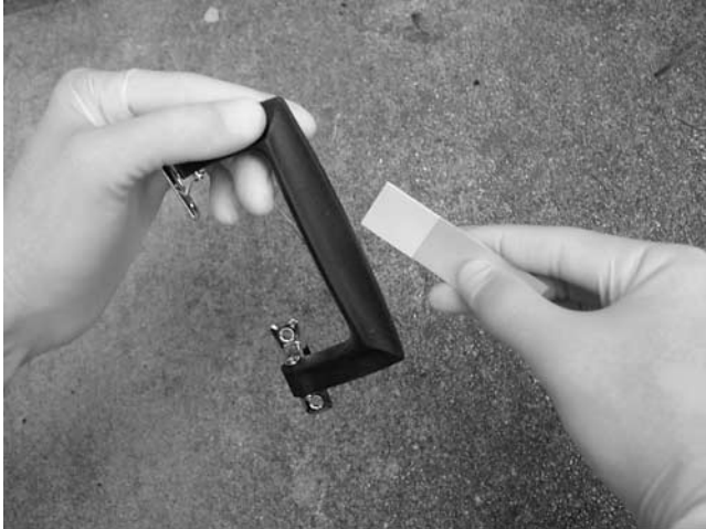
Figure 10. Dry transfer strip contaminating a handle.
