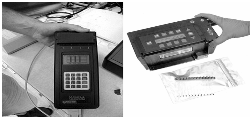
FIGURE 5-7 Handheld PCR devices. Two next generation fluorescent real-time PCR devices. On the left is the handheld advanced nucleic acid analyzer (HANAA), a prototype device developed by Lawrence Livermore Laboratories. The device is battery operable and has four cycling chambers to hold PCR reaction tubes. The unit on the right is Idaho Technology's RAZOR system, which cycles temperatures for the reaction by moving reaction mixtures back and forth in the plastic tubes between fixed temperature chambers and can run 12 reactions simultaneously. In each case, the nucleic acid has to be first extracted from the sample matrix before running the FRT/PCR. With the RAZOR system a set of prepackaged extraction reagents is provided in syringes, and the final sample is injected into the blue plastic receiver tubes. Photos courtesy of Jim Higgins (left) and Idaho Technology (right).
