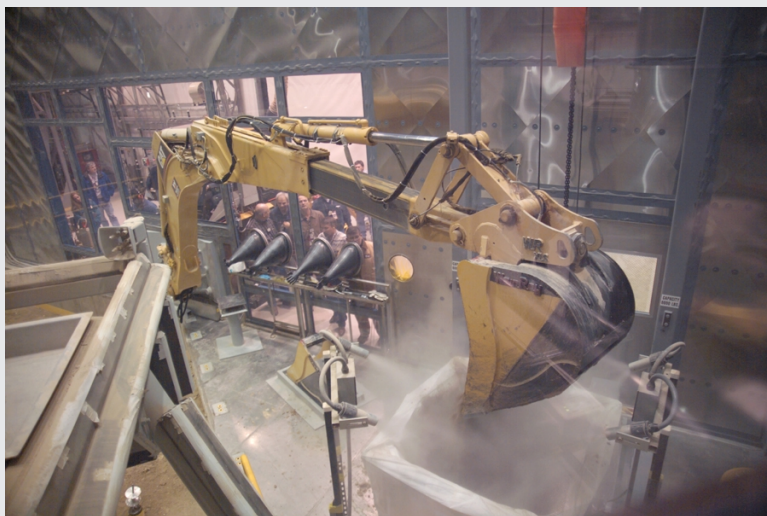
FIGURE 3.2 The glovebox excavator method (GEM) was a pilot project for retrieving waste at INEEL. While successful, it also demonstrated the cost and difficulty of retrieving some types of wastes at EM sites. Photo courtesy of INEEL.
