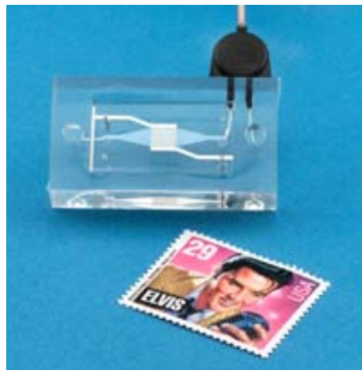
FIGURE 6.3 Photograph of hybrid microfluidic circuit that contains a commercial micropump (Mainz, Germany), a dielectrophoresis chip, load and waste wells, and fluidic interconnects, potted in silicone rubber.
