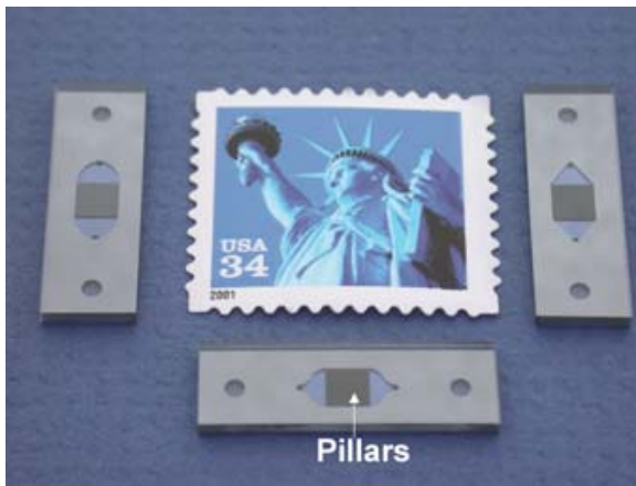
FIGURE 6.2 Arrays of microfabricated pillars with silica surfaces.
