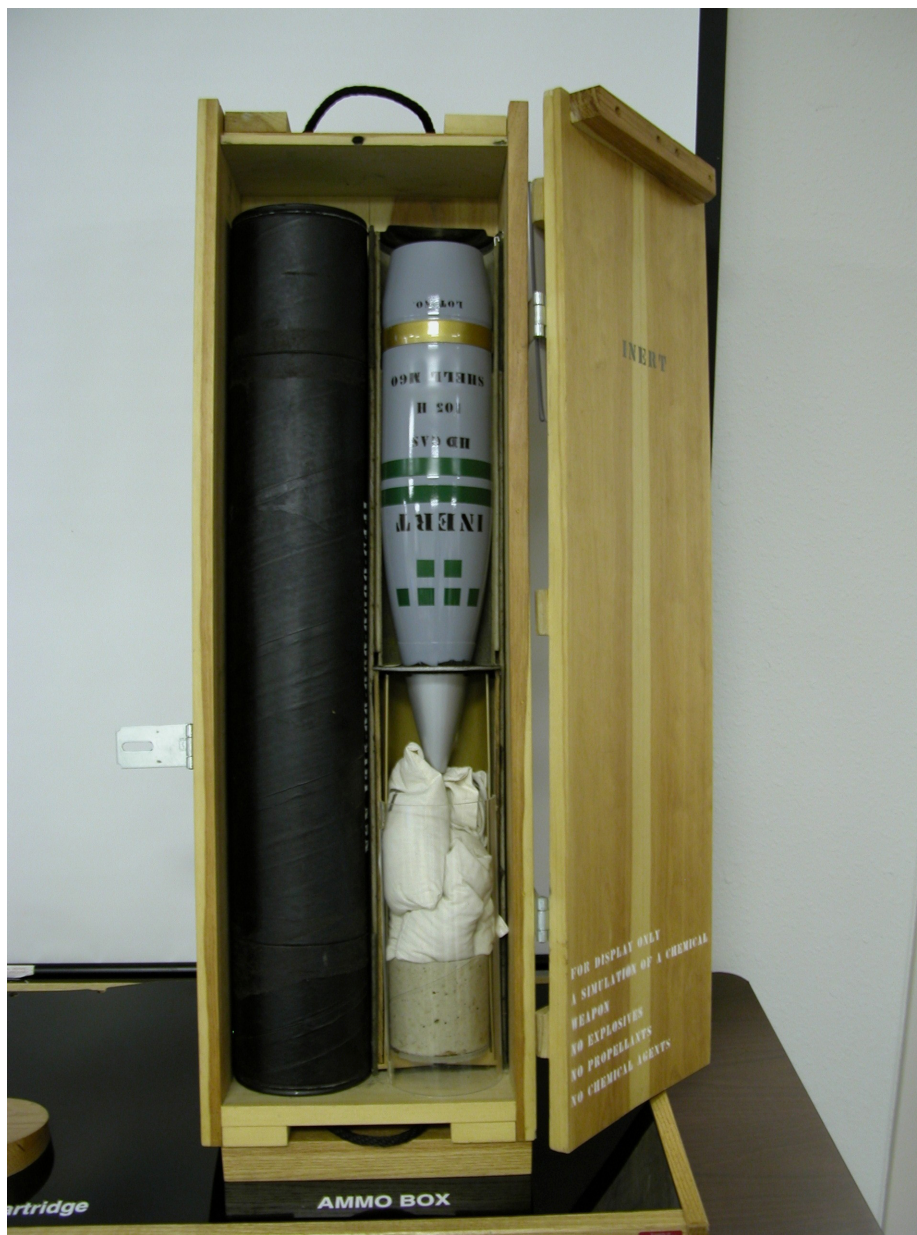
FIGURE A-4 Boxed 105-mm projectile showing the casing, the propellant bags, and other dunnage in the fiberboard tube. SOURCE: Personal communication from Yu-Chu Yang, Chief Scientist, Office of the Program Manager for Assembled Chemical Weapons Alternatives, Department of Defense, to Harrison Pannella, NRC staff, July 20, 2004.
