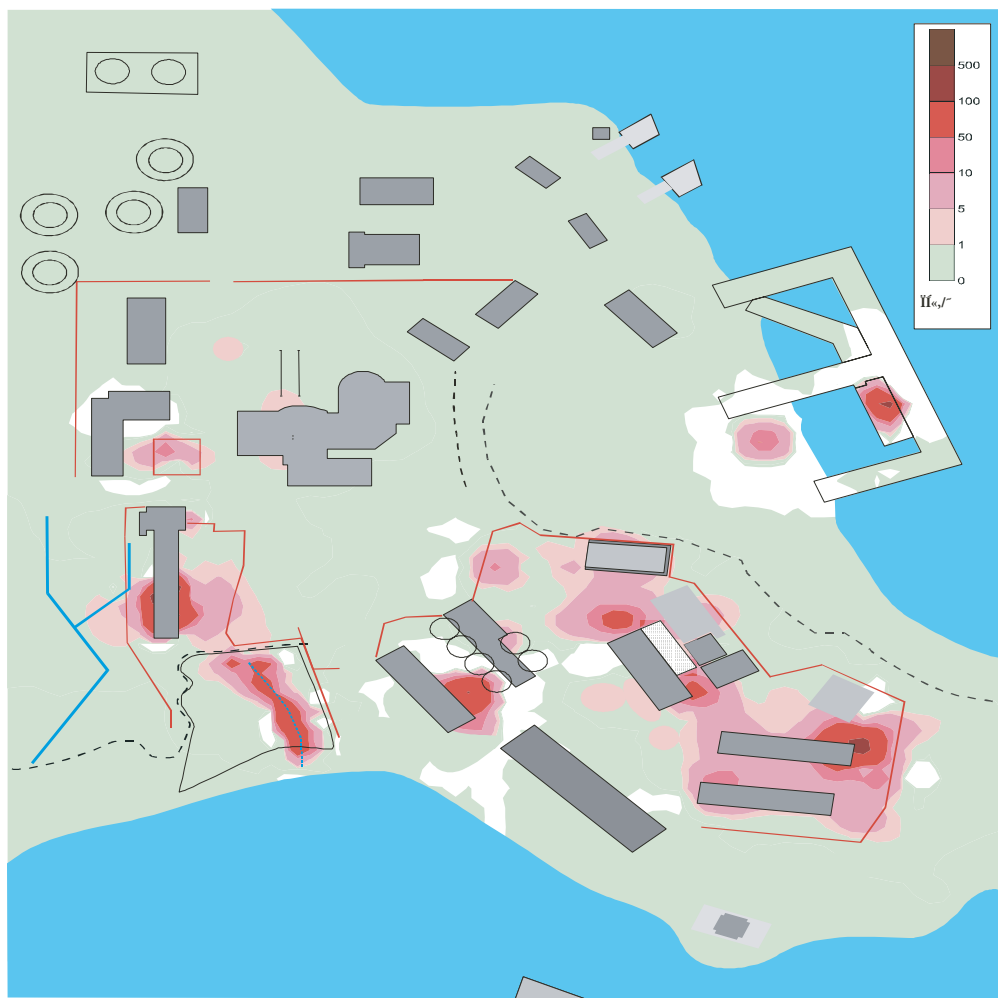
FIGURE 19 Dose rate at the Andreeva Bay base (at 0.1 m off the ground).
