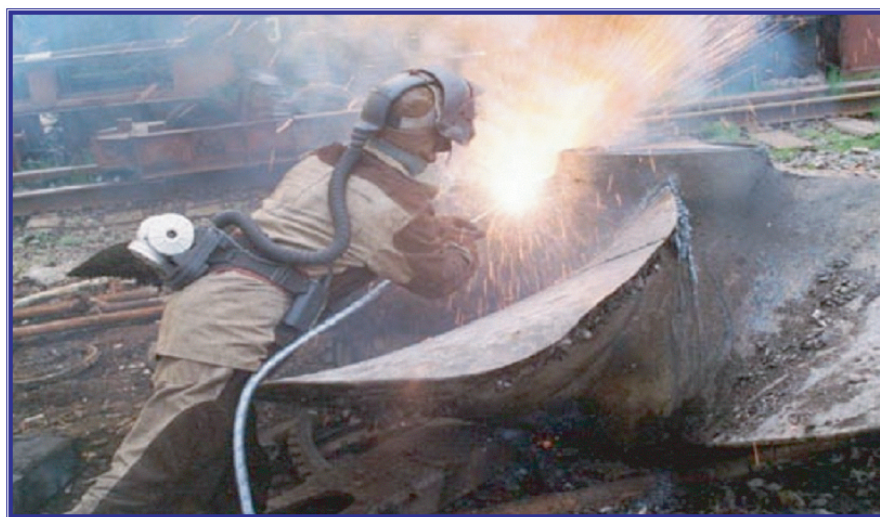
FIGURE 21 Severing of nuclear-powered submarines by gas cutting.
