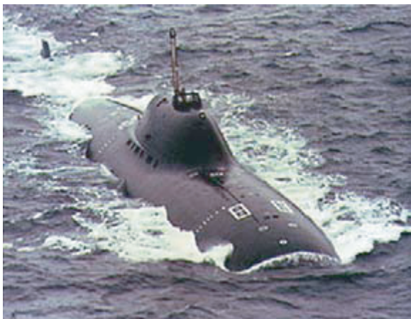
FIGURE 3 Nuclear-powered attack submarine with a liquid metal-cooled reactor (Alpha).
