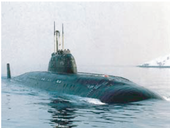
FIGURE 2 Nuclear-powered attack submarine with a water-moderated, water-cooled reactor (Victor II).
