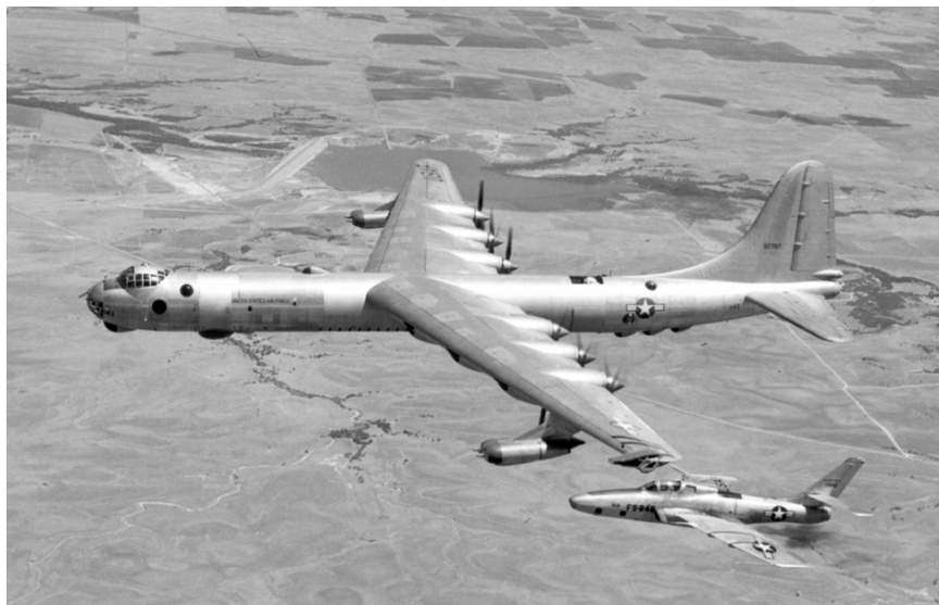
FIGURE 2.4 Project Tom Tom demonstrated drag savings from formation flight. SOURCE: Courtesy of the National Museum of the U.S. Air Force. Available online at < www.wpafb.af.mil/museum/history/postwwii/tomtom.htm >. Accessed June 2005.
