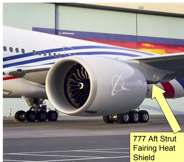
FIGURE 1-5 The aft strut fairing heat shield on the Boeing 777. This is currently designed using a titanium alloy and might be replaceable by a higher-temperature-capable PMC.
