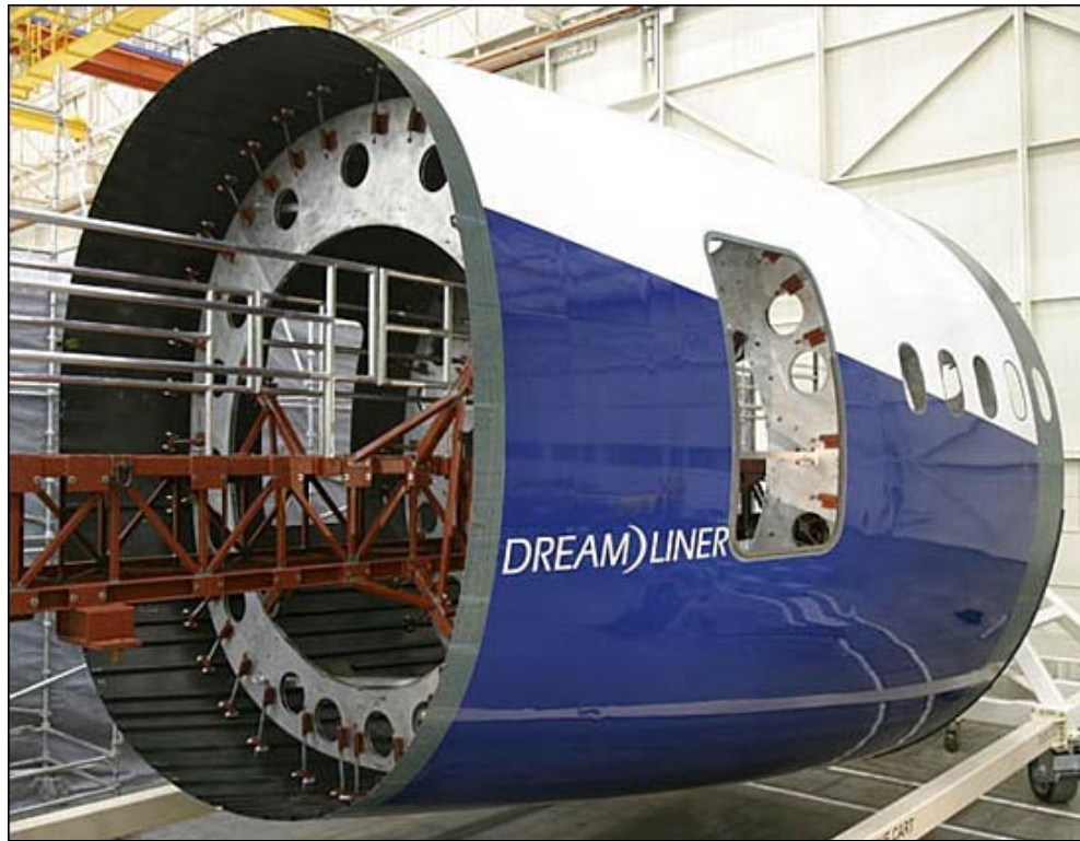
FIGURE 6-1 The Boeing 787 as designed will utilize composite materials and new manufacturing techniques, including building full barrel fuselage sections with integrated stringers, as shown here. This application of composite materials could result in fewer parts and improved aerodynamic performance and fuel efficiency.
