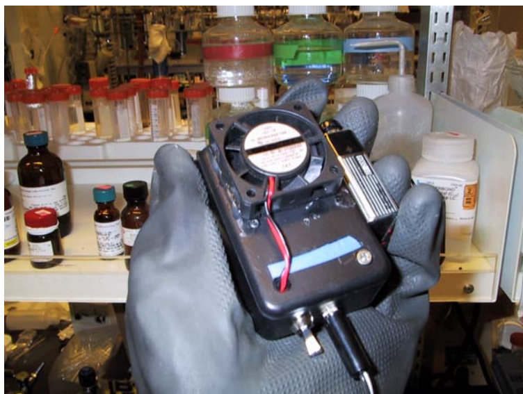
FIGURE 5-18 (Left) Handheld nanosensor device for nerve agent developed for the Micro Unattended Ground Sensors program (program manager: Edward Carapezza) of the Defense Advanced Research Projects Agency. The device contains a porous Si photonic crystal which contains chemistry that allows it to respond specifically to sarin (GB) gas. (Right) Testing run showing response to sarin at 10 ppm within 7 minutes of introduction. The sampling chamber was depleted of agent approximately 10 minutes into the run. SOURCE: Courtesy of M.J. Sailor, University of California, San Diego, and Kwok Ong, Aberdeen Proving Ground/Edgewood Arsenal.
