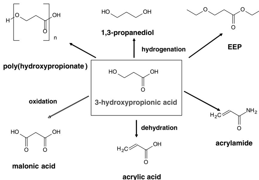
FIGURE 3.4 3-HP from sugar platform as a chemical building block.
