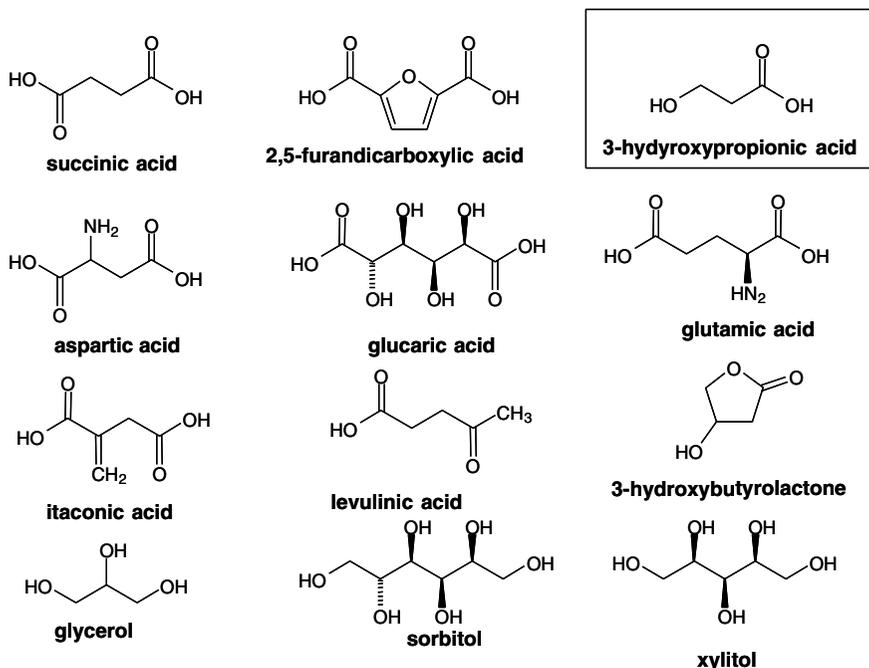
FIGURE 3.3 DOE biomass program “Top 12” sugar-based building block chemicals.
