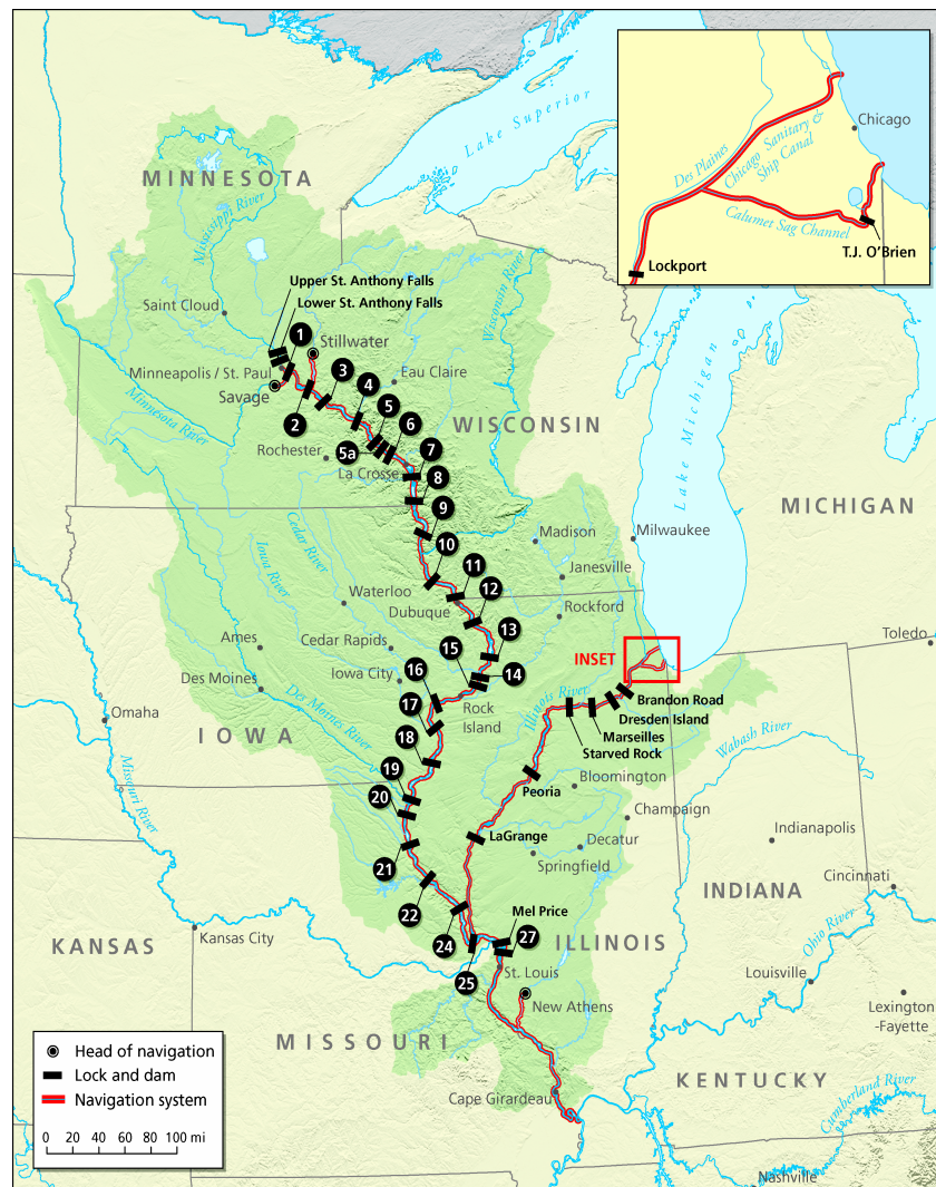
FIGURE 1.1 Locks and dams on the Upper Mississippi River-Illinois Waterway.
