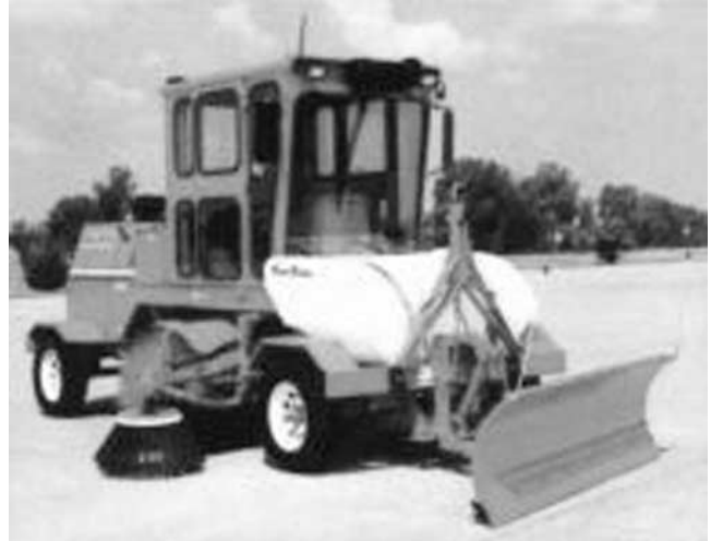
FIGURE 38 Typical rotary broom.
