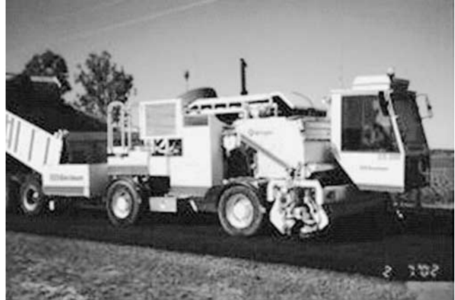
FIGURE 40 Low-drop aggregate spreader.
