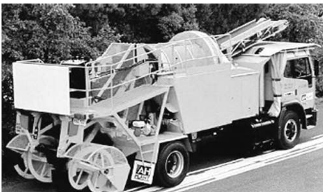
FIGURE 39 Aggregate precoating loader.
