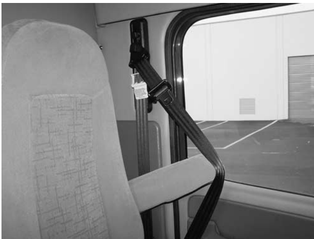
Figure 10. Shoulder strap tension adjustment mechanism (unlatched).
