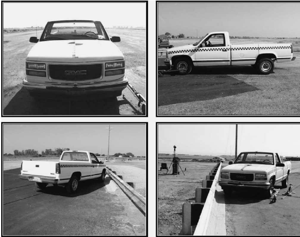
Figure 28. Test vehicle and setup for Type B curb beneath guardrail.
