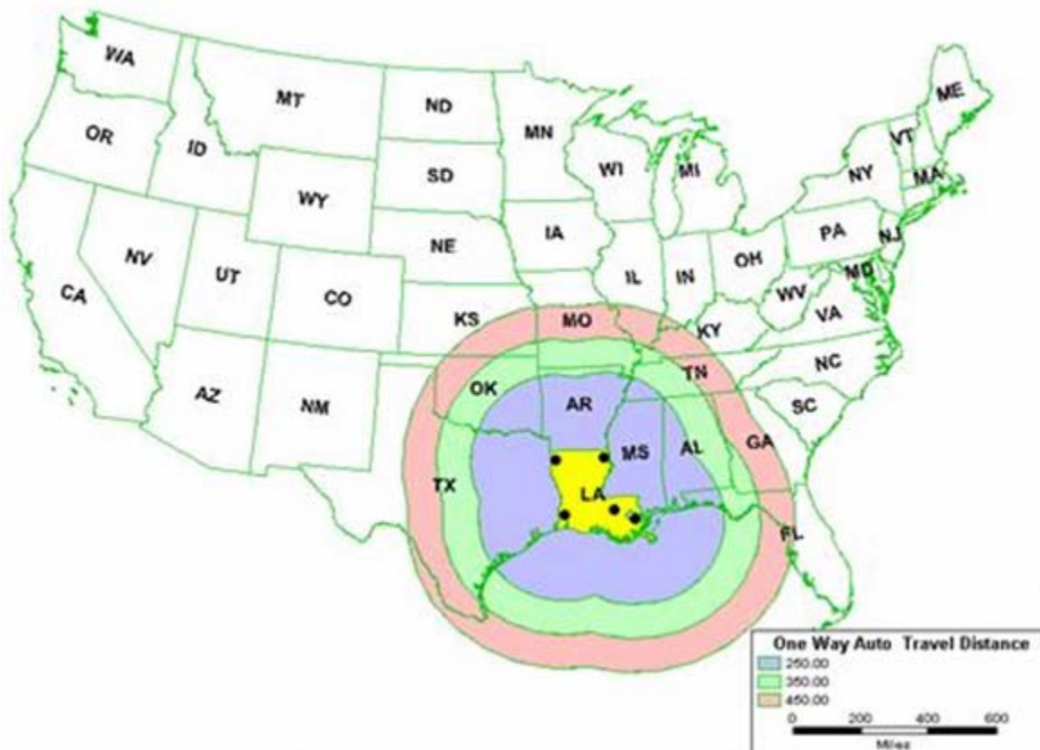
FIGURE 18 American Travel Survey—auto trip lengths to, from, and through Louisiana: 66% < 250 mi; 82% < 350 mi; and 90% < 500 mi.
