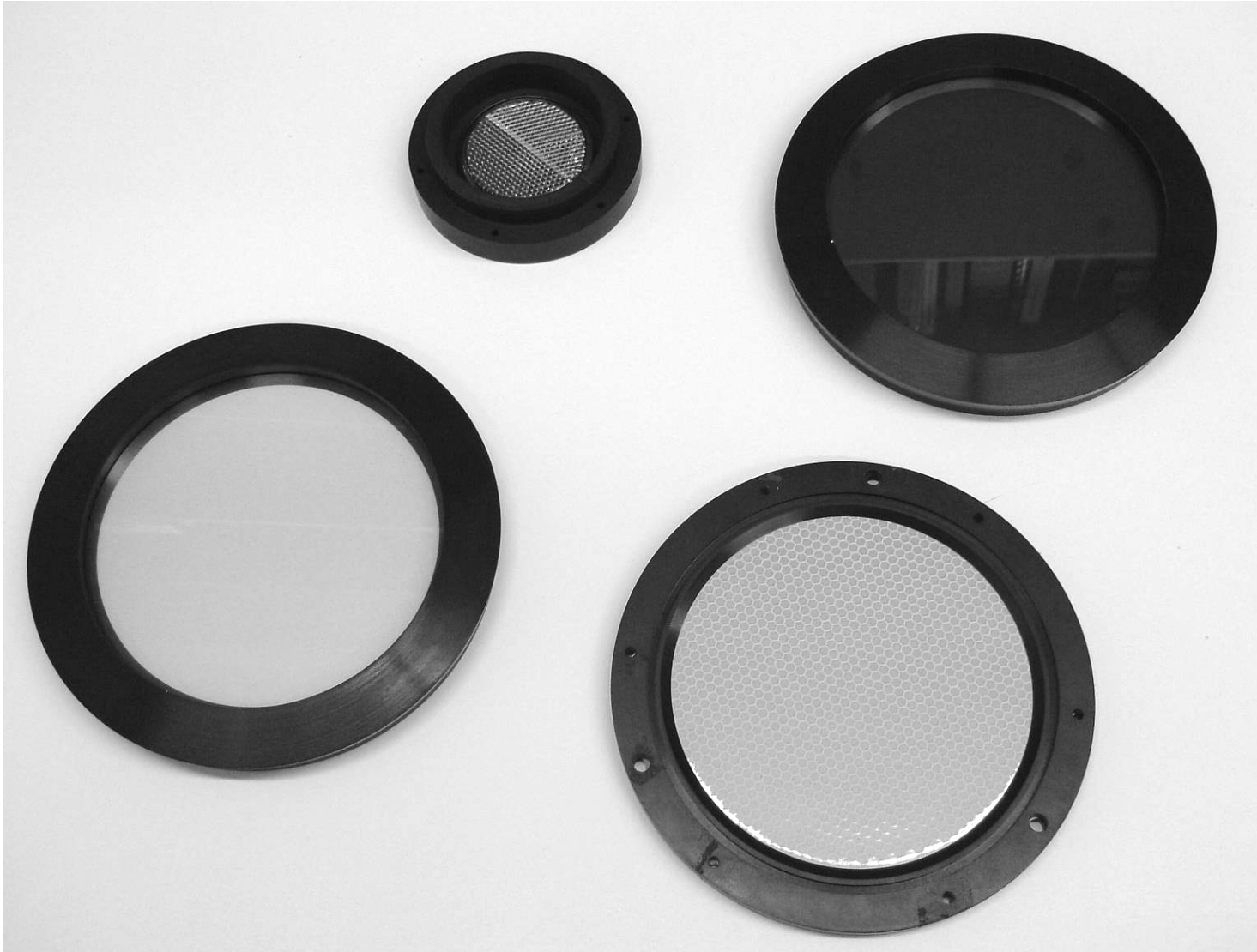
Figure 42 – Shown is the set of retroreflective samples used in the MAP service originally.
