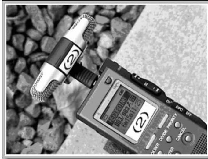
Figure 10—Image of stereo microphone recorder deployed outside of both tracks during study.
