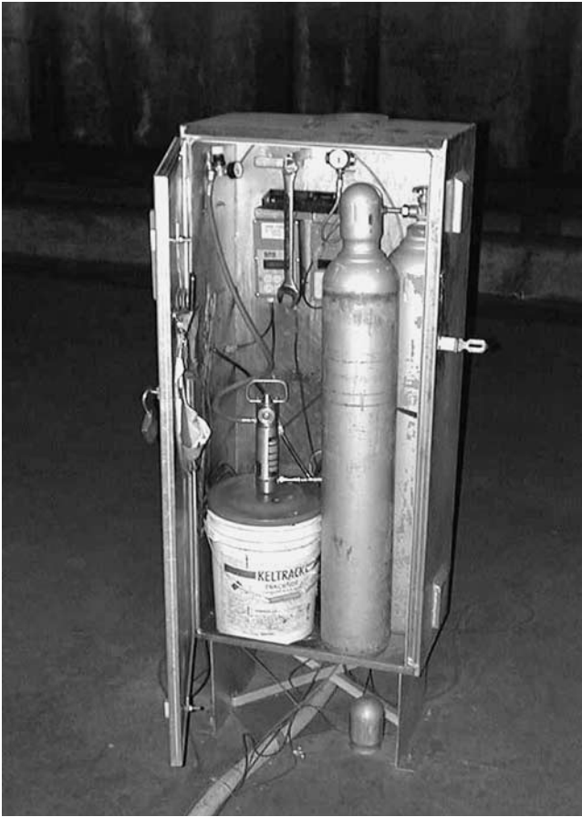
Figure 1. Nitrogen gas-charged lubricant/friction modifier cabinet.
