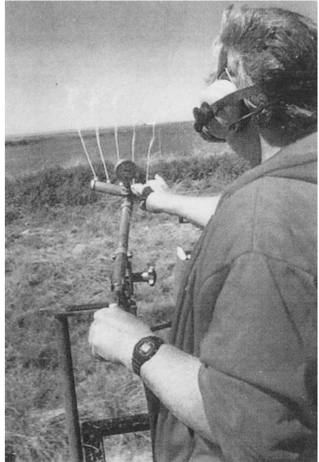
FIGURE 17 Field demonstration of invert-emulsion carriers shows good "targeting" several feet from the specialized nozzle manifold ( courtesy: Washington State DOT ).
