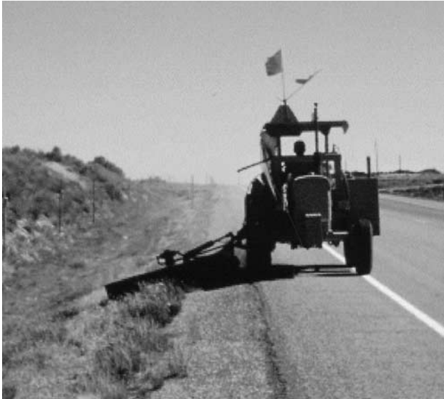
FIGURE 3 Mechanical control using a roadside mower in Idaho (courtesy: John Cantlon, E. I. DuPont Co.).
