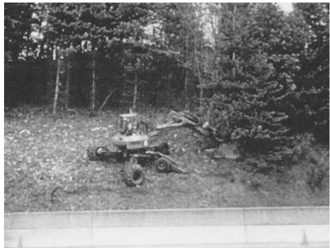
FIGURE 13 Specialized mowing equipment cuts brush and trees on steep slopes (courtesy: John Cantlon, E. I. DuPont Co.).
