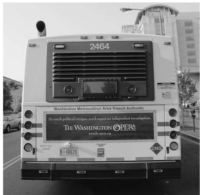
FIGURE 1 Rear of natural gas bus; blue CNG diamond is shown at the lower right.
