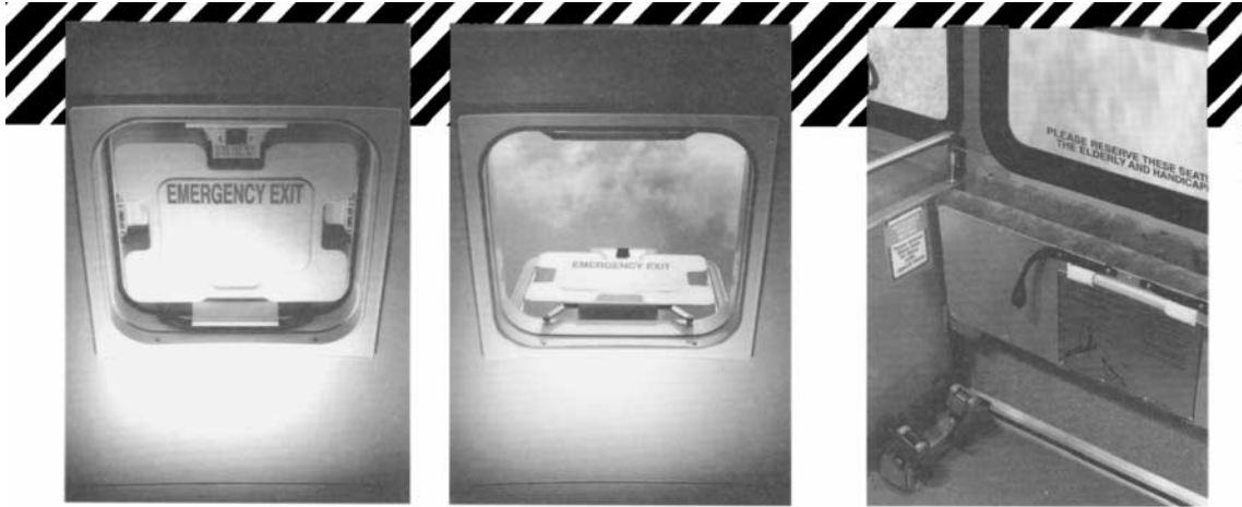
EMERGENCY ROOF HATCH Shown from inside the bus. PUSH black tab in direction shown PULL handle out.
