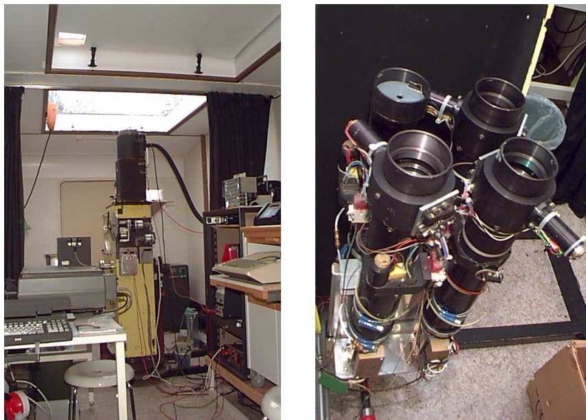
FIGURE 3.6 Instruments deployed in the field at Sandkullen, Sweden. Left: Ebert-Fastie spectrometer with an extremely high throughput that usually operates in the ultraviolet (instrument on loan from Johns Hopkins University). Right: A set of filter photometers that measure the atomic oxygen green line, molecular oxygen A-band, and hydroxyl radical Meinel band in the visible and near IR (as well as the scattered mercury green line at 540.6 nm and relevant continua). SOURCE: Stockholm University Department of Meteorology optical site at Sandkullen, Sweden. See < www.misu.su.se/~jacek/Ground/optsite.html >.
