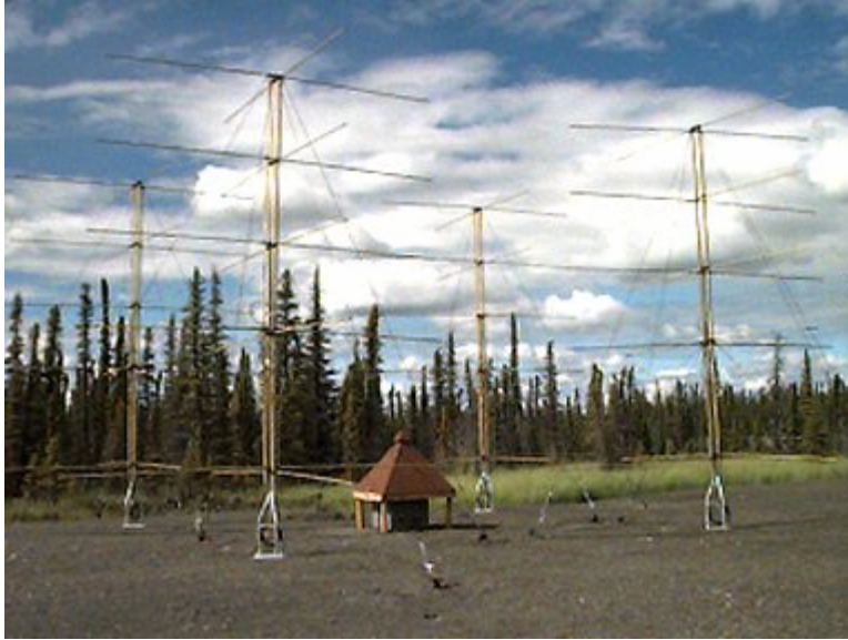
FIGURE 3.1 Photo of a riometer that employs a traditional or classic design. Shown here is the 30-MHz High Frequency Active Auroral Research Program (HAARP) riometer, which is part of a major ionospheric research facility located near Gakona, Alaska. This riometer uses a 2 \times 2 array of five-element yagi antennas and a low-noise receiver to achieve a very sensitive receiver capability. SOURCE: HAARP, Office of Naval Research and the Air Force Research Laboratory. Image available at www.haarp.alaska.edu/haarp/rioImages/rio.jpg .
