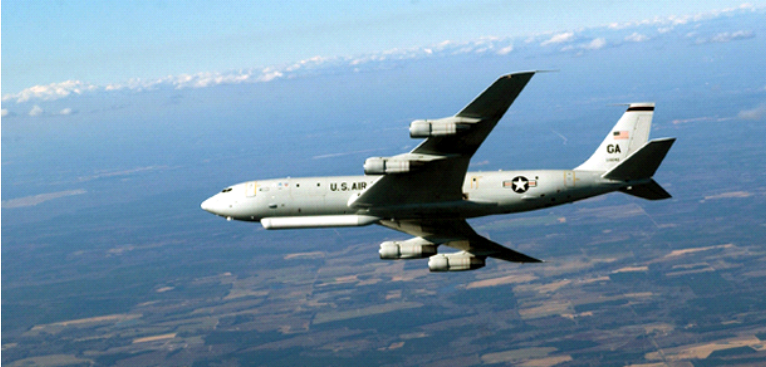
FIGURE D.8 E-8C Joint Surveillance Target Attack Radar System. SOURCE: Courtesy of the Department of the Air Force.
