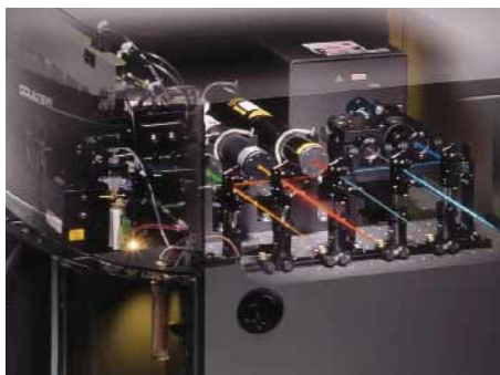
FIGURE 25 A color photograph of a flow cytometer showing the multiple colors of lasers.
