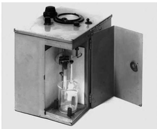
FIGURE 2 Arnold Beckman's first integrated pH meter, the acidimeter, circa 1934. Courtesy of Beckman Coulter, Inc.
