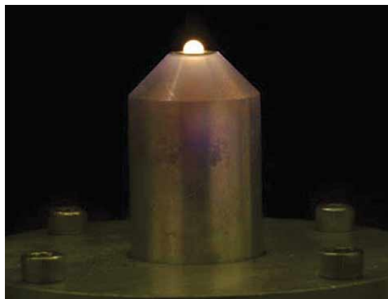
FIGURE 17 Novel sample environments enable research into matter under extreme conditions within Earth. Inelastic x-ray scattering from levitated (containerless) molten alumina at high temperature is used to gain information on the liquid dynamics within Earth's mantle. The levitated liquid aluminum oxide sample in a supercooled state at approximately 1800°C is shown.
