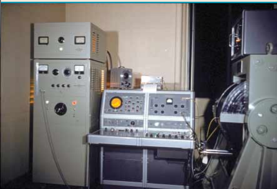
FIGURE 6 40-MHz console, magnet, and power supply (1954).
