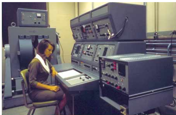
FIGURE 11 The DFS-60 NMR spectrometer, the first routine ^{13}\text{C} instrument, used time averaging. Photo taken in 1966.
