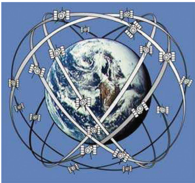
FIGURE 2-5 Schematic drawing of the Global Positioning System (GPS) constellation. The GPS uses 24 satellites (21 plus spares) at an altitude of about 11,000 miles, moving at about 7,000 mph. A GPS receiver on Earth synchronizes itself with the satellite code and measures the elapsed time since transmission by comparing the difference between the satellite code and the receiver code. The greater the difference, the greater the time since transmission. Knowing the time and the speed of light, the distance can be calculated. The time comes from four atomic clocks on each satellite. The clocks are accurate to within 0.003 seconds per 1,000 years. Using information from four or more satellites, the GPS receiver calculates latitude, longitude, and altitude. SOURCE: National Aeronautics and Space Administration.
