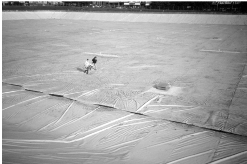
Preparing to sample stored drinking water from the access hatch of a floating cover on a distribution system reservoir. Photo courtesy of Bureau of Laboratory Service, Philadelphia Water Department.
