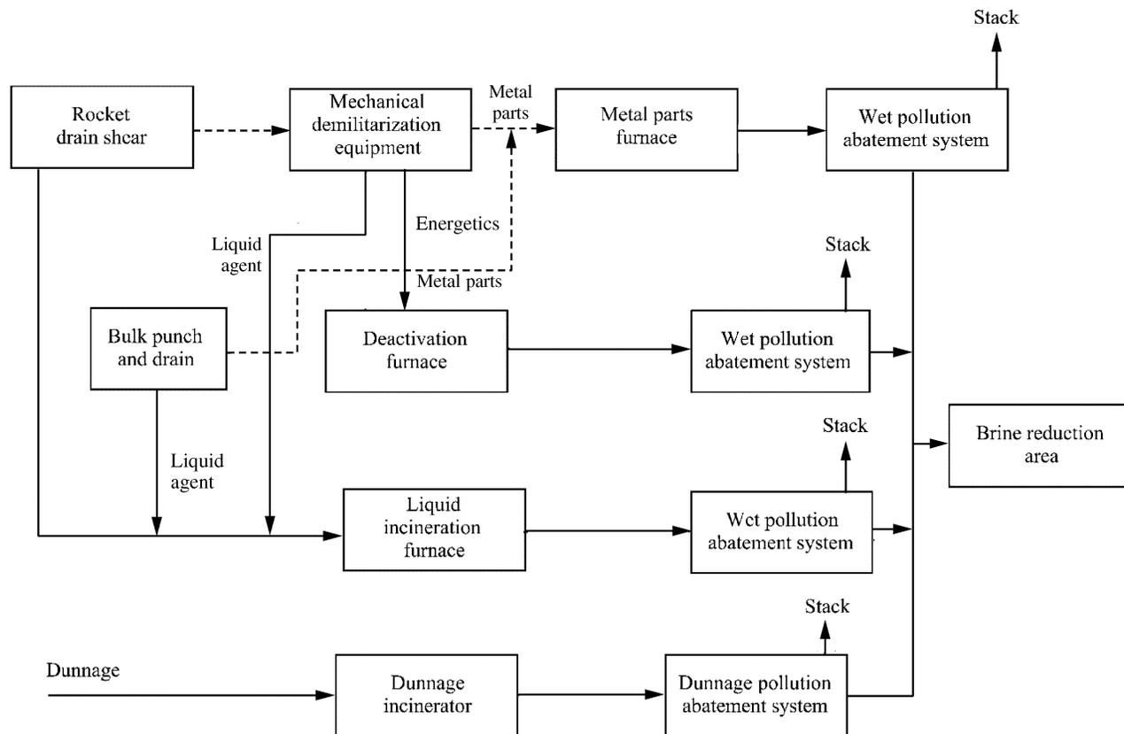
FIGURE 5-4 Block diagram of U.S. baseline incineration system. SOURCE: Pearson and Magee, 2002.
