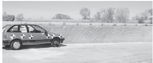
Figure 33. Caltrans single-slope barrier with fluted surface texture.
