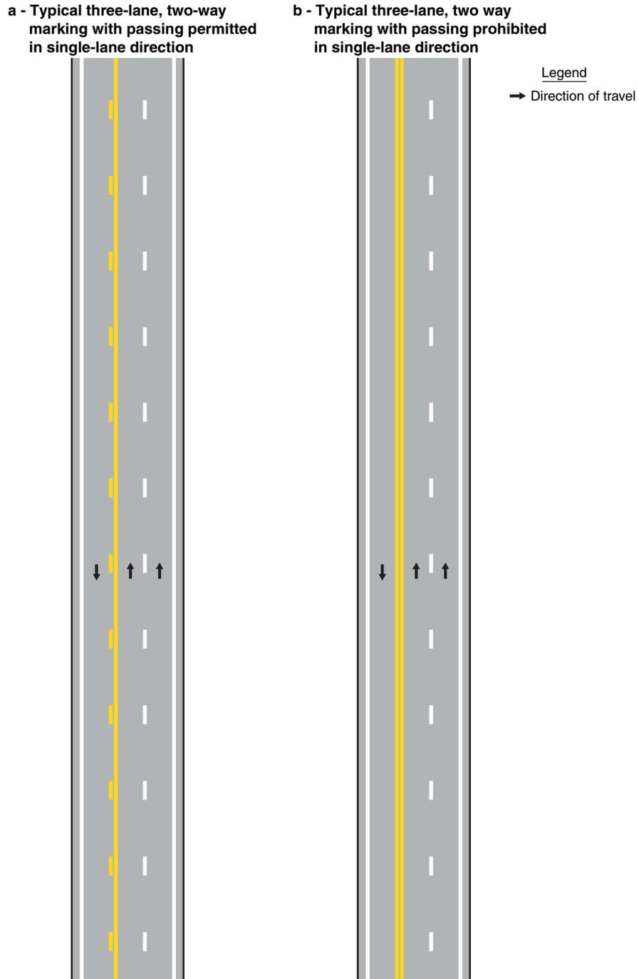
FIGURE 3B-3 Examples of Three-Lane, Two-Way Marking Applications
