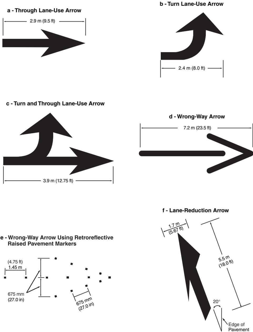
Typical sizes for normal installation; sizes may be reduced approximately one-third for low-speed urban conditions; larger sizes may be needed for freeways, above average speeds, and other critical locations. A narrow elongated arrow design is optional. For proper proportion, see the Pavement Markings chapter of the "Standard Highway Signs" book (see Section 1A.11).
