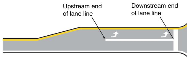
FIGURE 1 Illustration of terms upstream and downstream.
