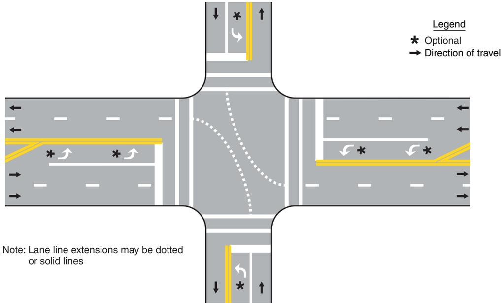
**d - Typical dotted line markings to extend longitudinal centerline markings**
