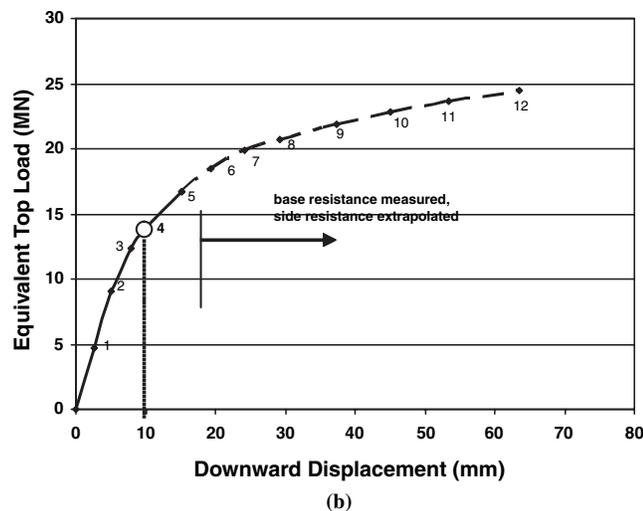
FIGURE 65 Construction of equivalent top-loaded settlement curve from O-cell test results (a) O-cell measured load-displacement; (b) equivalent top-load settlement results.
