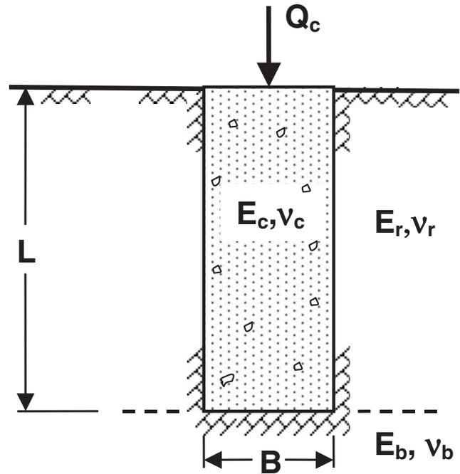
FIGURE 34 Axially loaded rock socket, elastic analysis.
