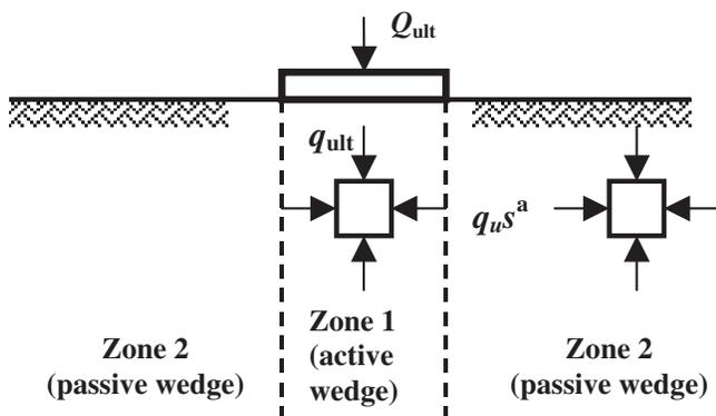
FIGURE 30 Bearing capacity analysis.
