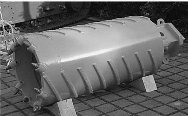
FIGURE 53 Typical single wall core barrel.
