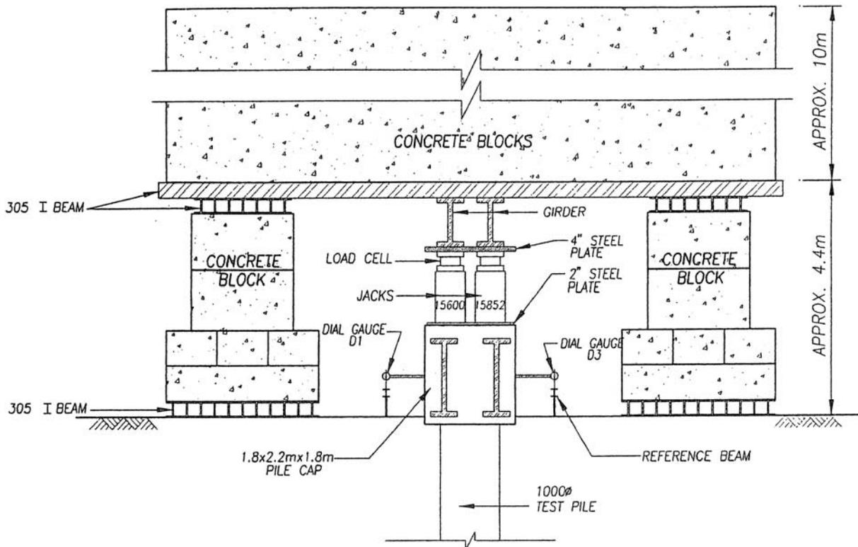
FIGURE 58 Axial load testing setup (Zhan and Yin 2000).
