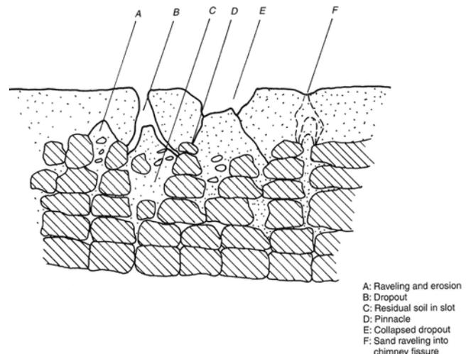
FIGURE 79 Features of karstic terrain (Knott et al. 1993).
