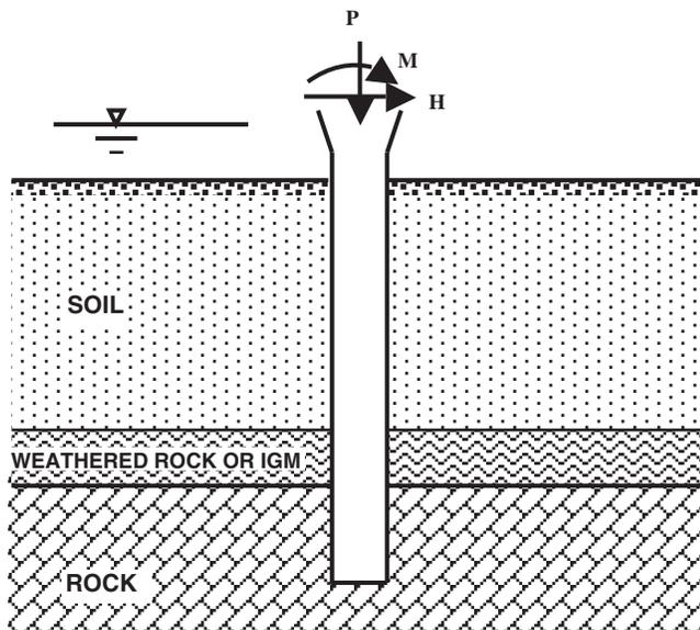
FIGURE 1 Rock-socketed shaft designed for highway bridge structure.
