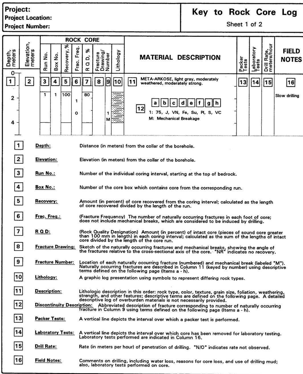
FIGURE 11 Key for rock core description (sheet 1).
