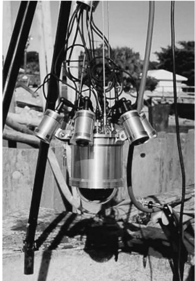
FIGURE 78 Shaft inspection device or SID.
