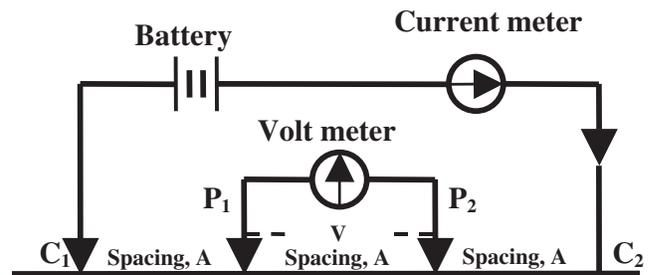
FIGURE 7 Field configuration for resistivity test.
