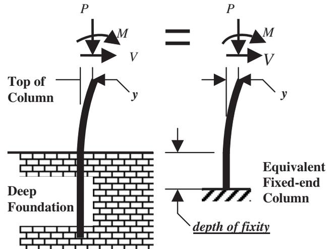
FIGURE 47 Depth of fixity for equivalent fixed-end column.
