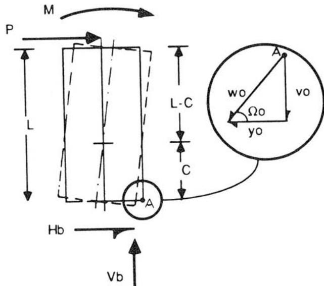
FIGURE 43 Base deformation as a function of shaft rotation (Gabr and Borden 1988).
