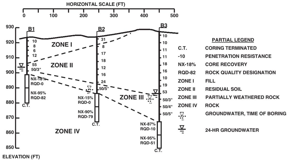
FIGURE 81 Typical Piedmont subsurface profile (after Schwartz 1987).
