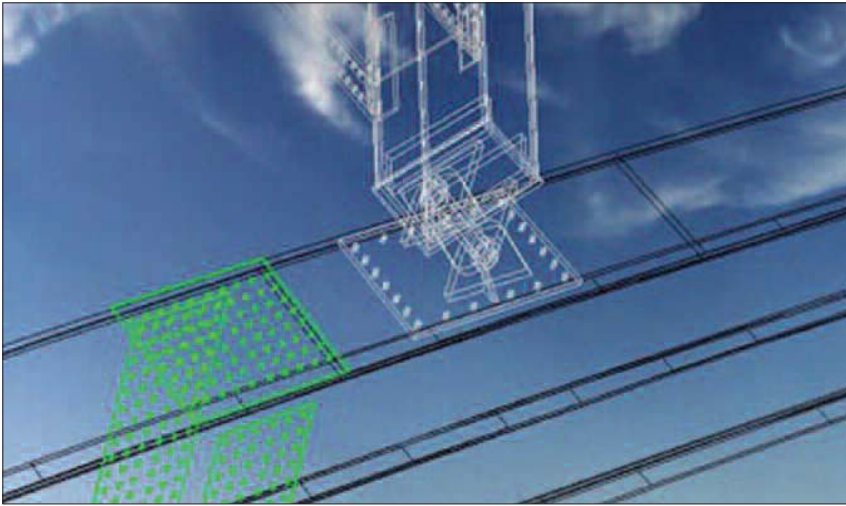
▲ A wireframe view of the main arch with column and splice connection.
