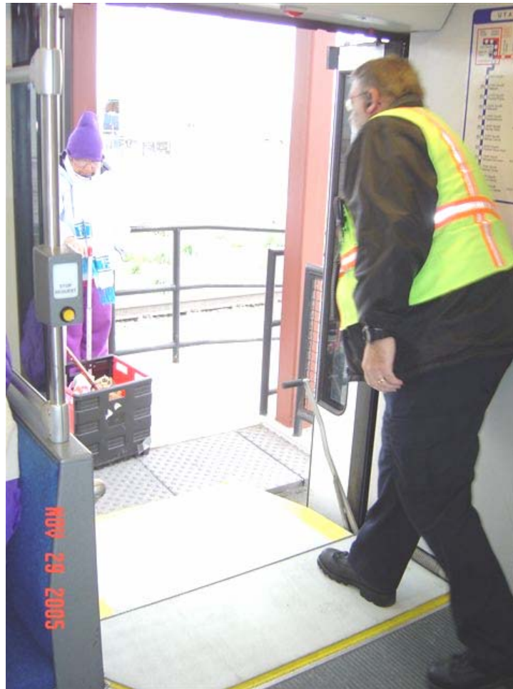
FIGURE 3 An operator lowers the bridgeplate to allow access for a disabled passenger to the vehicle.
