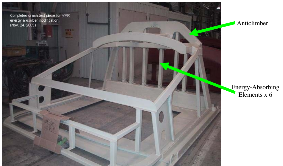
FIGURE 5 Controlled collapse cab structure prior to crash test.
