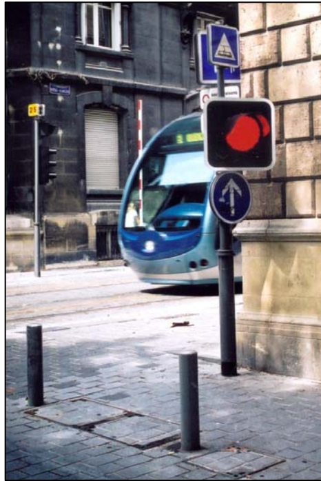
FIGURE 18 Post-mounted flashing red light signal assembly (regulatory), Bordeaux, France (urban environment, pedestrian mall operation).
