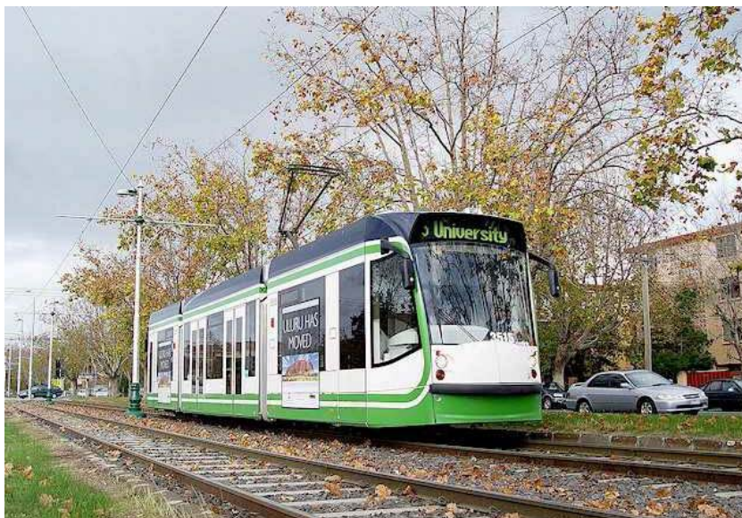
FIGURE 1 Melbourne tram on exclusive alignment.
