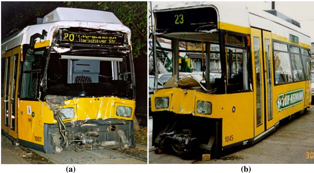
FIGURE 7 Comparison of vehicle damage produced by the collision: (a) Vehicle 1007 (GT6) and (b) Vehicle 1045 (GT6).
