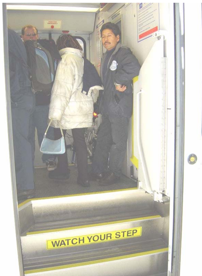
FIGURE 2 Passengers board a train at a door where the access ramp is not being used and the bridgeplate is locked in the up position.
