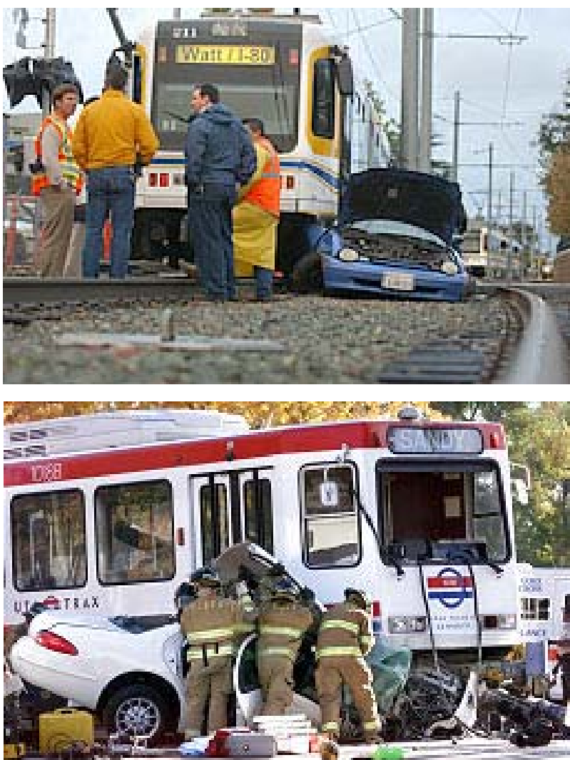
FIGURE 3 Override collision behaviors between LRVs and automobiles (13, 14).
