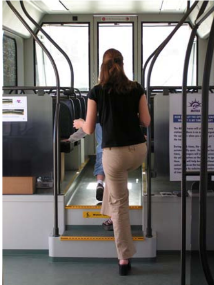
FIGURE 8 Transition from low- to high-floor area.
