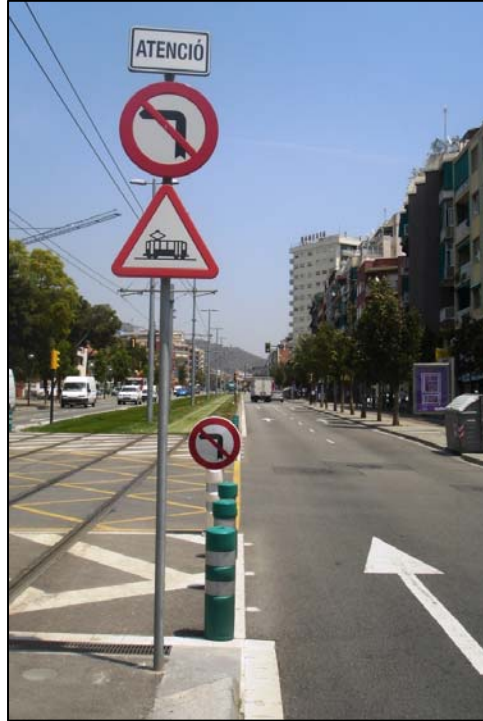
FIGURE 14 Left-turn prohibition (regulatory and warning) devices, Barcelona, Spain (urban environment, median operation).
