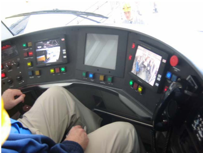
FIGURE 13 Ergonomic cab with video monitoring.
