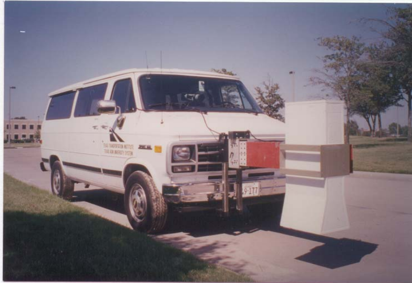
(a) TTI GPR Equipment
