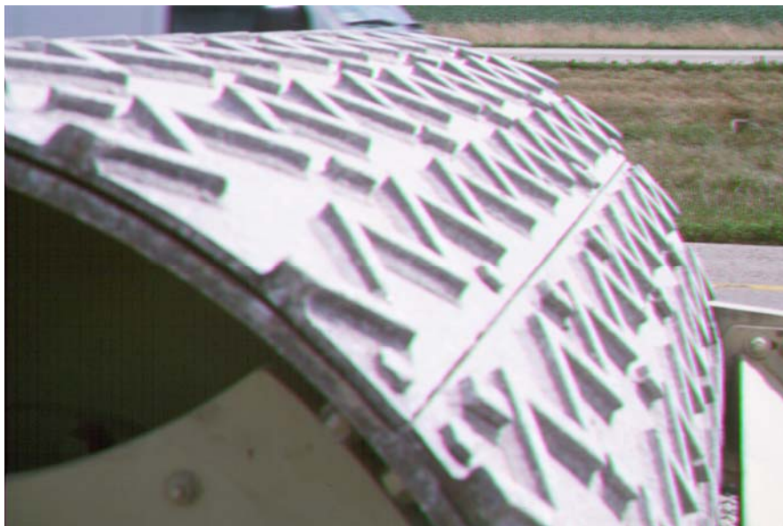
FIGURE 9 Roller with Elliott Grid. (Photo courtesy of Antigo Construction.)
