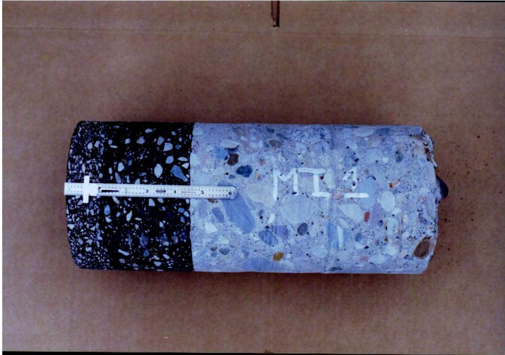
**Figure C44. Core of Pavement Structure, MI-1**
