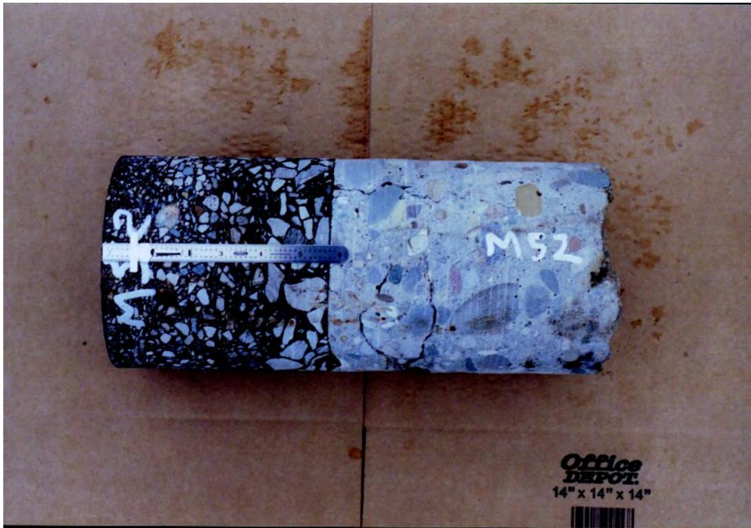
**Figure C46. Core Showing Pavement Structure, MI-3 Note Cracking in Concrete**
