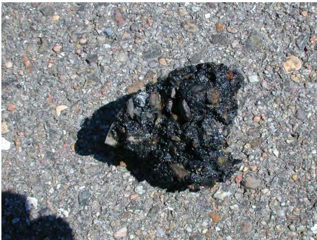
**Figure C37. Visual Evidence of Moisture Damage in Underlying Layer KS-1.**
