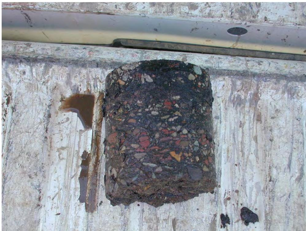
**Figure C17. Gooey Black Substance on Core, CO-2 Highway 82**
