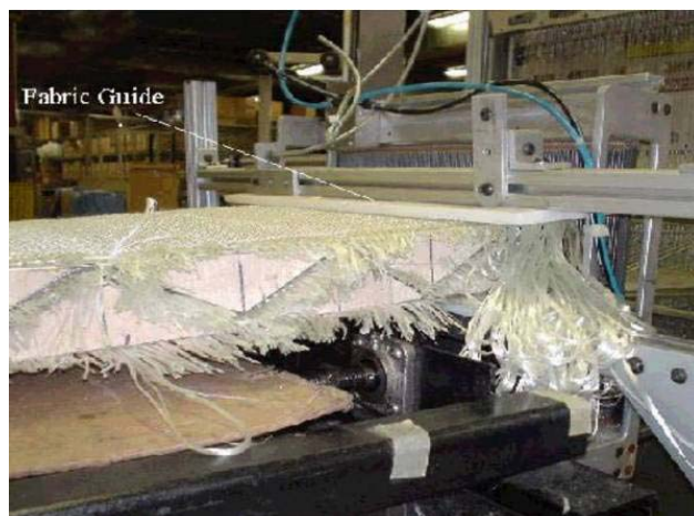
FIGURE 26 Three-dimensional weaving of a prototype glass fiber bridge deck.
