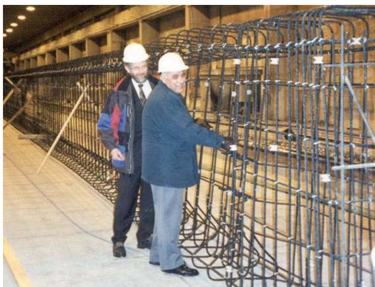
FIGURE 2 CFRP stirrups for prestressed girders.
