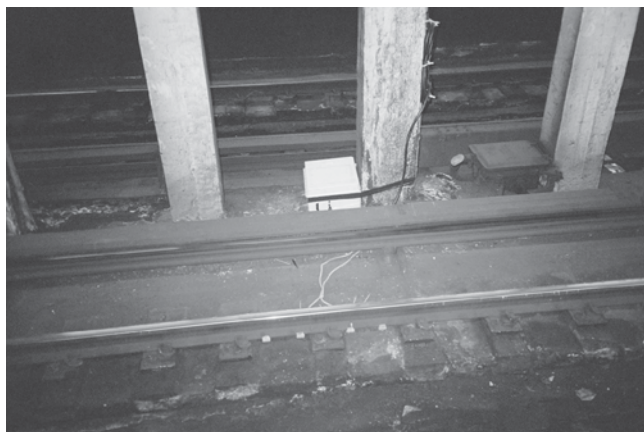
Figure 4 View of the transmitter case, which was subsequently mounted to one of the center pillars.
