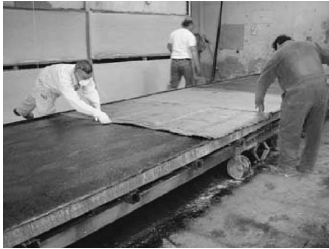
3.5.1-1 Hand lay-up operation: dry filament placement.
