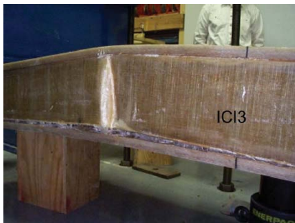
Figure 5.2.2.2-2 Example of web failure and debonding of thick facesheet from core.
