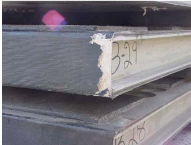
Figure 4.4.5-1 Exposed fiberglass fibers from installation damage.
