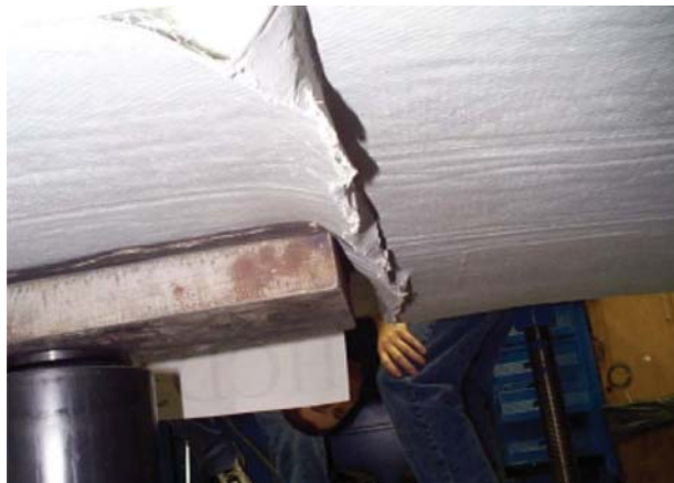
Figure 5.2.2.1-8 Example of thin facesheet crippling on foam sandwich deck.
