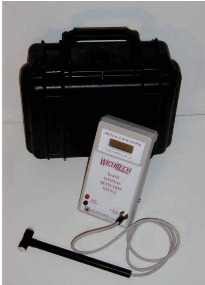
5.1.2-1 Electronic tap-tester unit.
