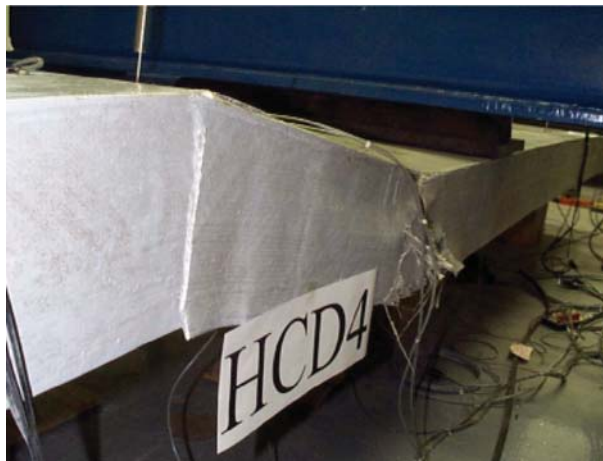
Figure 5.2.2.2-1 Foam sandwich deck failure under line load.
