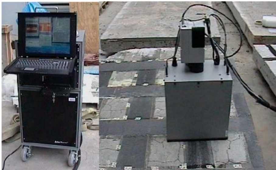
Figure 5.1.3-2 Thermal wave image processing unit and IR camera/heat source provide high resolution of local area.
