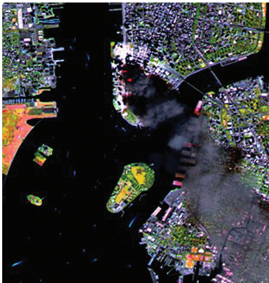
FIGURE 6.6 SPOT multispectral image with 20-m resolution taken 87 minutes after the collapse of the North Tower of the World Trade Center and 110 minutes after the collapse of the South Tower, clearly showing the particle plume transport to the southeast. Approximately 3 km from the source, the visible plume is about 1 km wide. SOURCE: Courtesy of SPOT Image Corporation, 2007.
