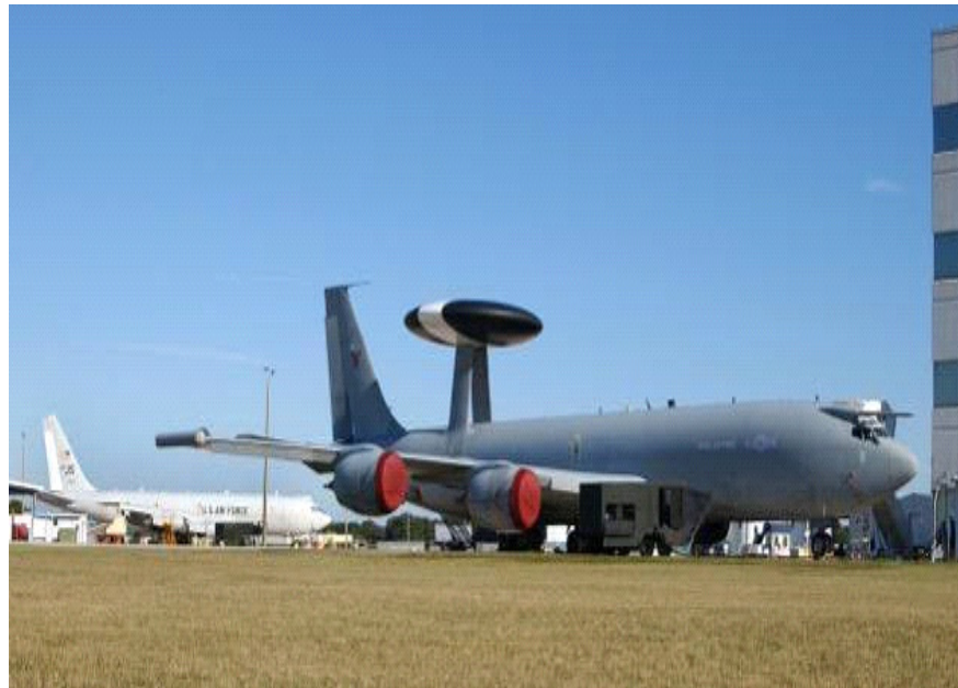
FIGURE 4-7 United Kingdom E3-D powered by GE/CFMI CFM56-2 engines. SOURCE: Alan van Weele.
