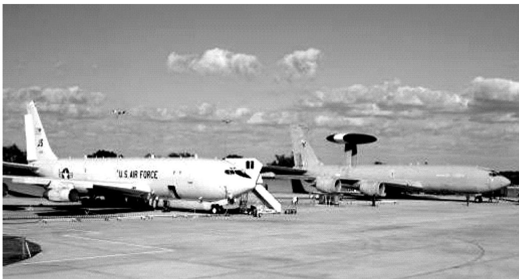
FIGURE 4-1 E-8 JSTARS with TF33-102C engines and Royal Air Force AWACS with CFM56-2 engines. SOURCE: Alan van Weele.
