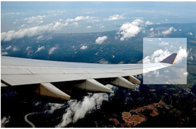
FIGURE 3-8 Airbus A340 with swept, canted winglets. SOURCE: Reproduced by permission of EADS North America.
