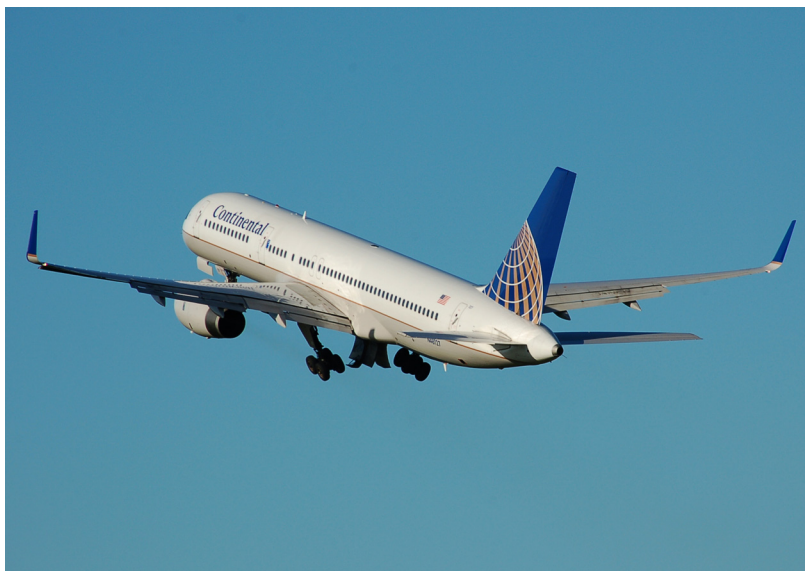
FIGURE 3-3 Boeing 757 with retrofit blended winglets. SOURCE: Courtesy of Adrian Pingstone.
