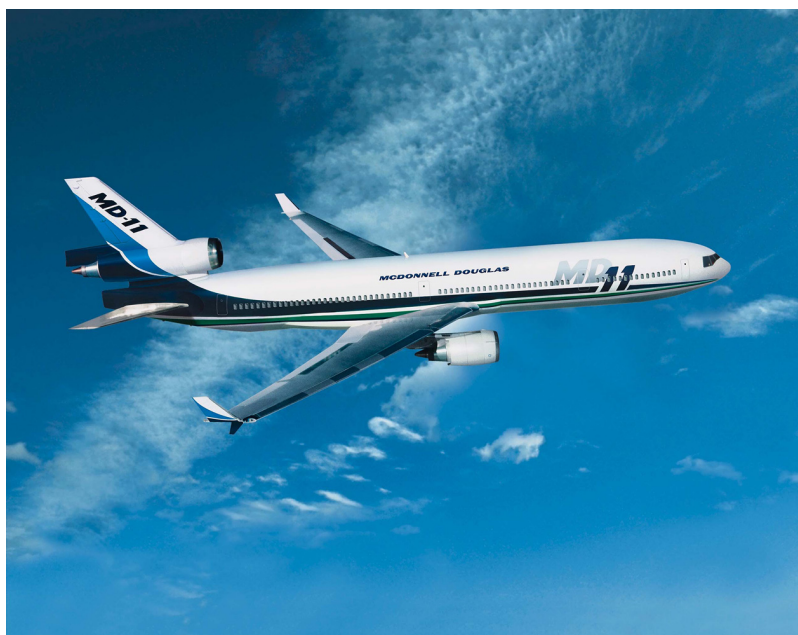
FIGURE 3-6 McDonnell Douglas MD-11 with dual winglets. SOURCE: Reproduced by permission of Boeing.
