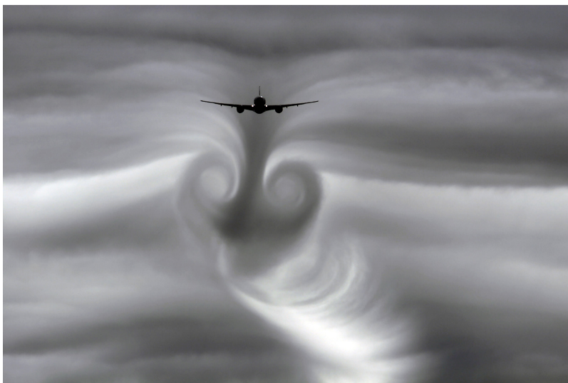
FIGURE 2-2 The vortex wake behind lifting wings descending through a thin cloud layer. SOURCE: Airliners.net . Photo courtesy of S.C. Morris.
