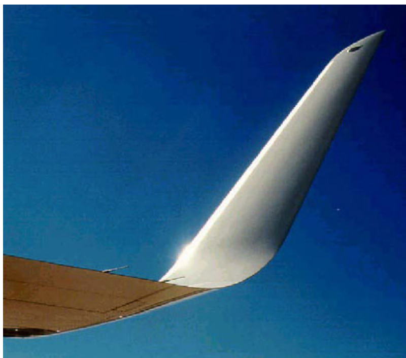
FIGURE 1-1 A common wingtip modification is the “winglet.” SOURCE: Aviation Partners Boeing (APB).
