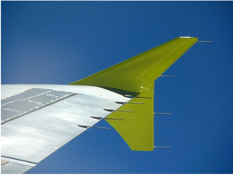
FIGURE 3-7 Airbus A320 with tip fence. SOURCE: Reproduced by permission of EADS North America.
