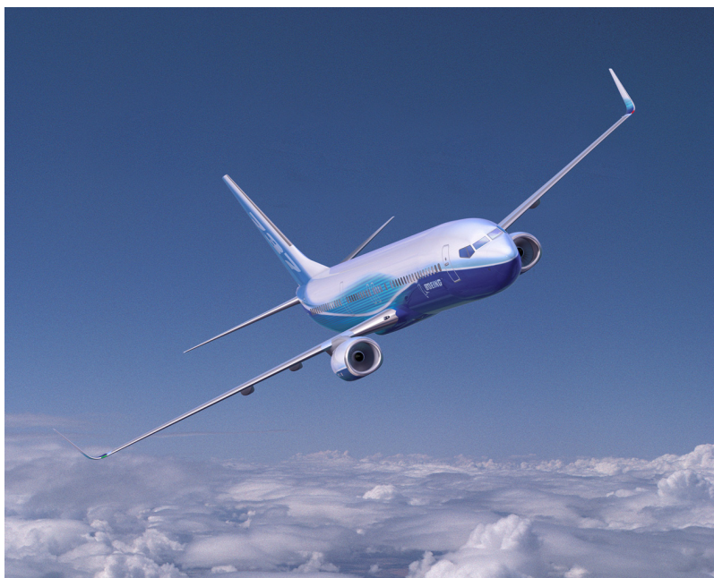
FIGURE 3-2 Boeing 737-NG with blended winglets. SOURCE: Reproduced by permission of Boeing.
