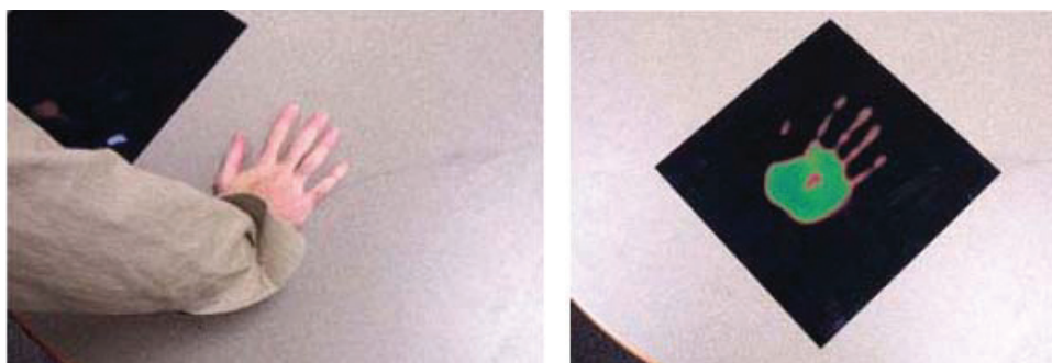
FIGURE C-13 Images showing the thermal response of a cholesteric liquid crystal. At room temperature, the device is black (upper left in the left frame). Heating by a hand causes changes in the observed color (right frame). SOURCE: Adapted from the University of Wisconsin-Madison IPSE Liquid Crystal Activity Guide < http://mrsec.wisc.edu/Edetc/supplies/ActivityGuides/LC_Activity_Guide_Expo.pdf >, Materials Research Science and Engineering Center on Nanostructured Interfaces, University of Wisconsin-Madison.
