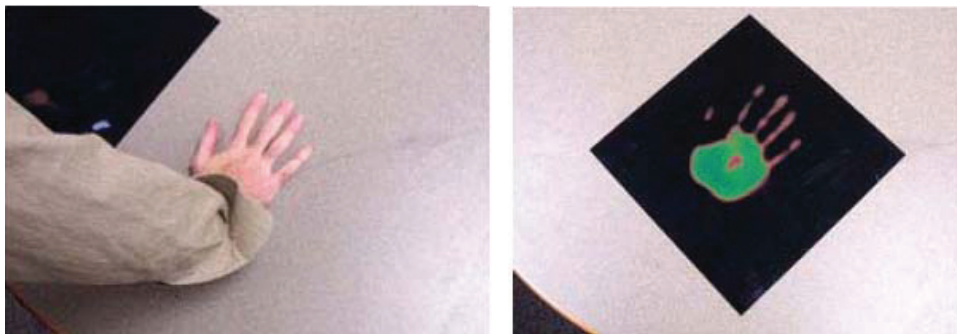
FIGURE 4-2 Images showing the thermal response of a cholesteric liquid crystal. At room temperature, the device is black (upper left in the left frame). Heating by a hand causes changes in the observed color (right frame). SOURCE: Adapted from the University of Wisconsin-Madison IPSE Liquid Crystal Activity Guide; < http://mrsec.wisc.edu/Edetc/supplies/ActivityGuides/LC_Activity_Guide_Expo.pdf >.
