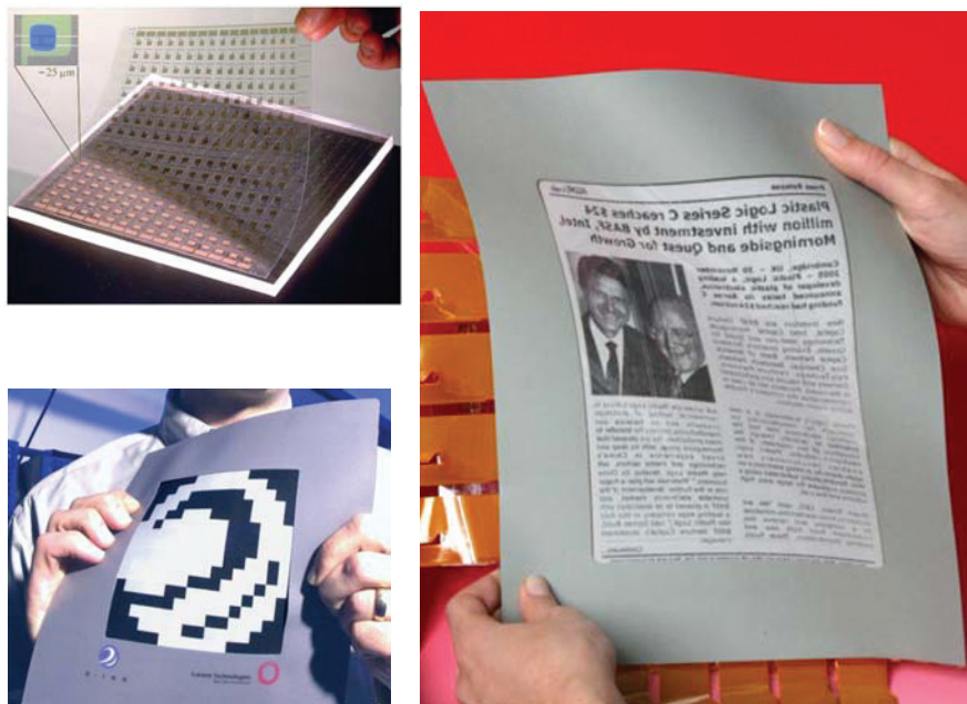
FIGURE D-7 Flexible, paperlike displays that integrate electrophoretic inks with printed flexible electronic backplane circuits. The images show (top left) an initial demonstration and (bottom left) a printed backplane circuit (Rogers et al., 2001); and (right) an example of the current state of the art (< http://www.plasticlogic.com >).
