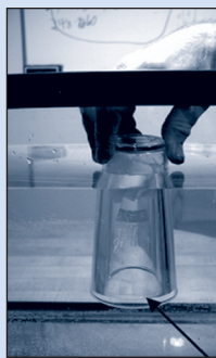
FIGURE 3-5 Fully submerged glass: only a small amount of water gets in.
