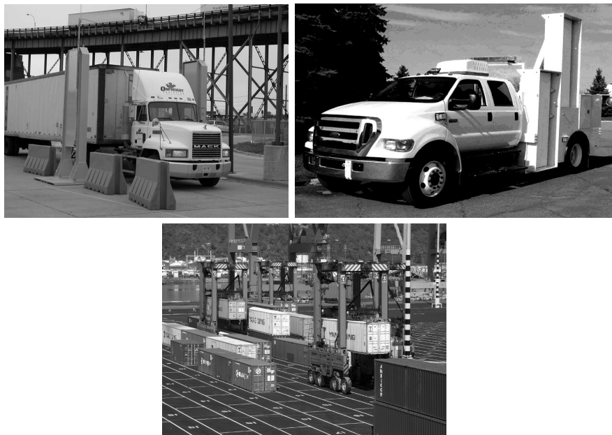
FIGURE 5-4 Standard truck exit RPM system (left), mobile RPM system (middle), and straddle carrier operation (right).
