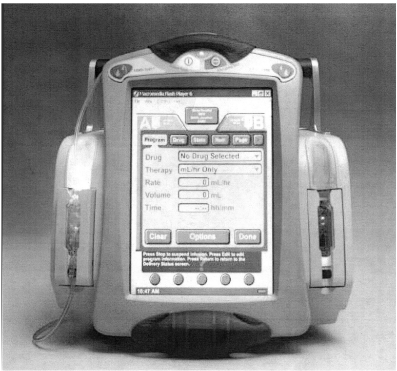
FIGURE 5-5 Two channel IV pumps with left channel illuminated. Photograph courtesy of Hospira, Inc.
