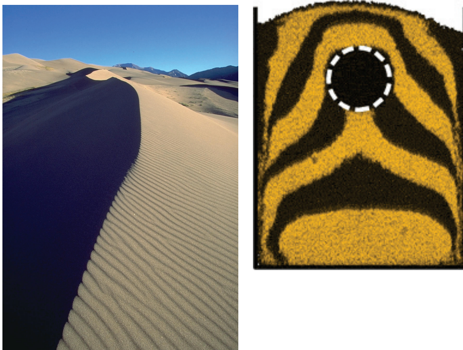
FIGURE 1.4 Granular materials consist of individual solid grains interacting only at contact, yet large assemblies of such grains exhibit a rich set of complex behaviors. (Left) Ripples in a sand dune. (Right) While fluids mix when stirred, granular materials size-separate; this magnetic resonance image of the interior of a layered granular system shows the upward motion of a large particle (dotted circle) in a bed of smaller ones. SOURCES: (Left) Photo courtesy of http://philip.greenspun.com . (Right) Matthias Möbius and Heinrich Jaeger, University of Chicago.
