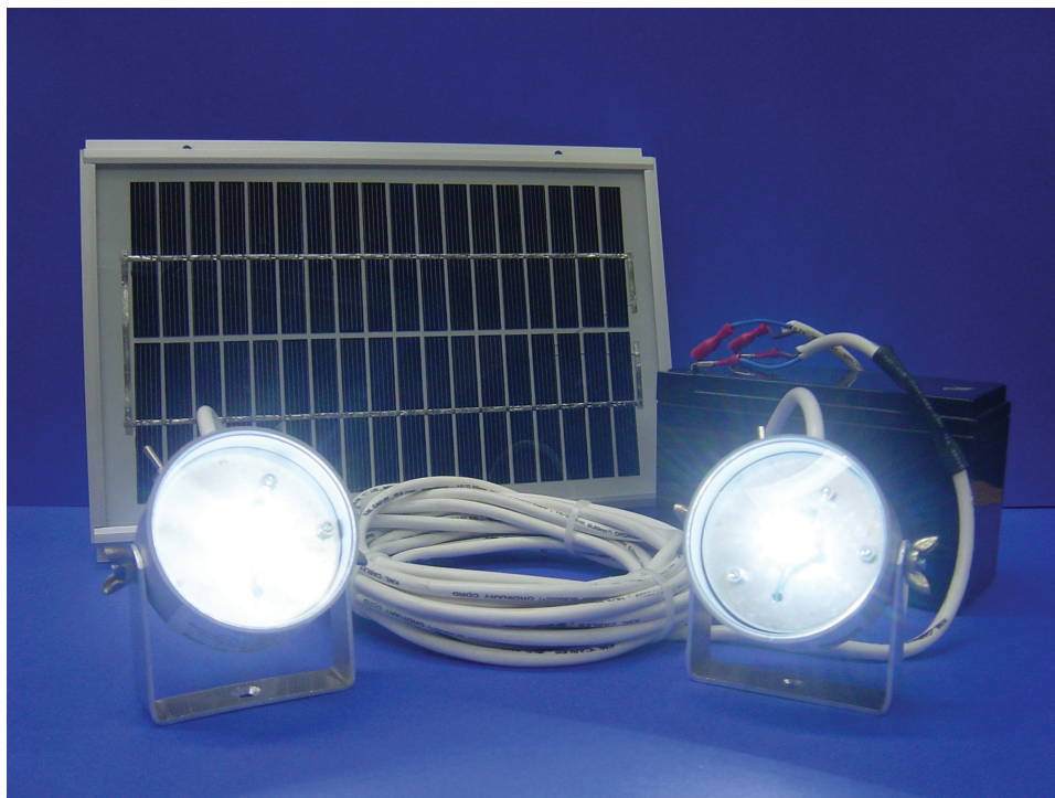
FIGURE 3.4 Applications of solid-state lighting in developing countries. The system comprises two modular 1-watt white light-emitting diode lamps; a 12-volt, 7-ampere-hour sealed lead acid battery (rechargeable and maintenance free); and a 5-watt solar panel. The system has a 100,000-hour lifetime. SOURCE: Courtesy of Light Up the World Foundation.
