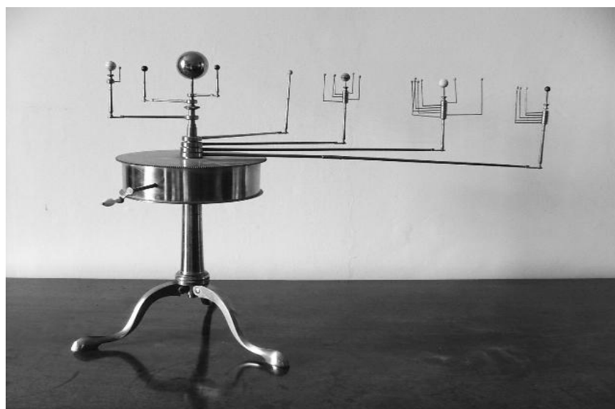
FIGURE 1-3 An orrery or physical model of the solar system. Source: C. Mollan, National Inventory of Scientific Instruments, Royal Dublin Society. Image courtesy of Miruna Popescu. Reprinted with permission; copyright 2004, Armagh Observatory.
