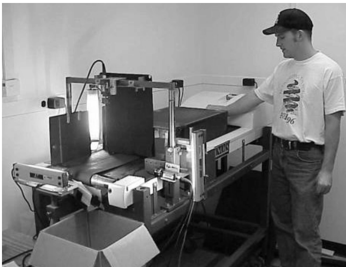
Figure A-3-4. Photo of the UIAIA system with operator passing aggregate particles.
