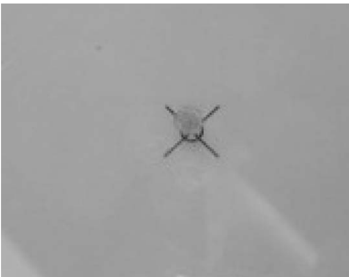
Figure A-1-12. Close-up view of Mylar sheet over light table. (Note: objects in photo appear misaligned due to parallax error. Look straight down on light table to achieve the optimum alignment.)
