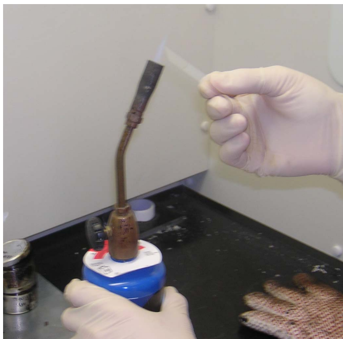
Figure B-2. Glass Slide Dried Before Immersion by Passing it Over a Propane Flame.
