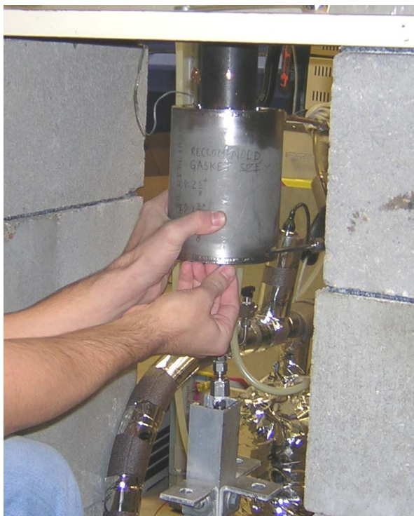
Figure C-5. Temperature Jacket Raised to Cover Adsorption Cell.
