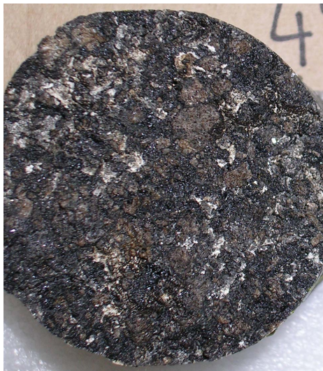
Figure I.5. Failure Plane of Moisture Conditioned Sample after Dynamic Creep Test.
