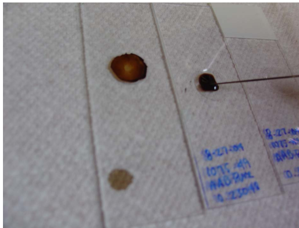
Figure G.2. Solvent Cast Procedure where a 0.025 mL Aliquot of a 0.0578 \pm 0.0002 g (asphalt/mL) Toluene is Deposited onto a 12.5 mm Diameter Glass Disc Slide.
