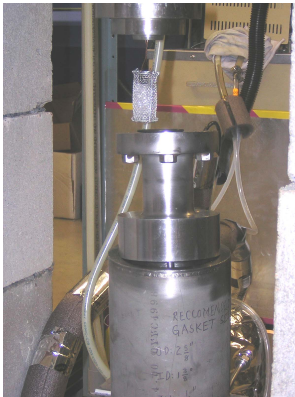
Figure C-3. Sample Basket Suspended from the Magnetic Suspension Balance.
