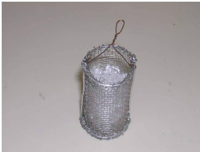
Figure C-2. Basket with Aggregate Sample for Testing with the USD.
