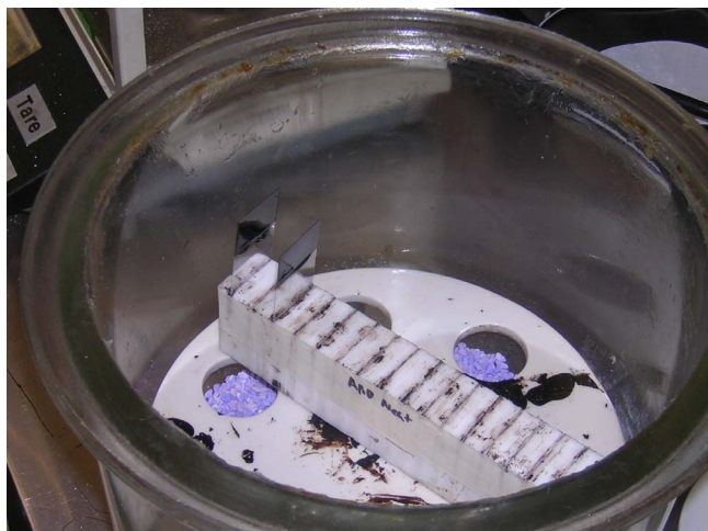
Figure B-5. Finished Slides Stored on Slotted Holder in Desiccator Prior to Testing.
