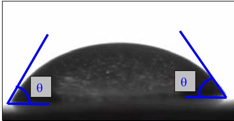
Figure 32. Typical Image of Sessile Drop for Contact Angle Measurement.
