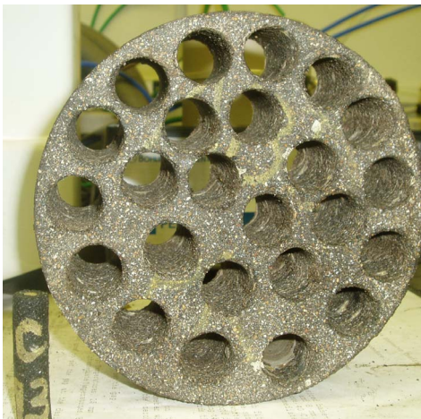
Figure I.7. SGC Compacted Sample and 12 mm Sample for DMA Testing.
