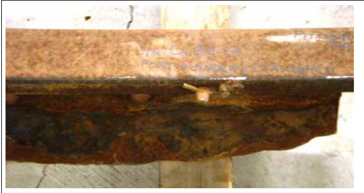
*Rail donated by PAAC showing severe corrosion at the base.*
