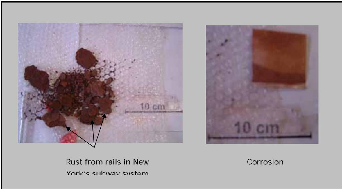
*Figure D8. Corrosion products found in New York's subway system.*
