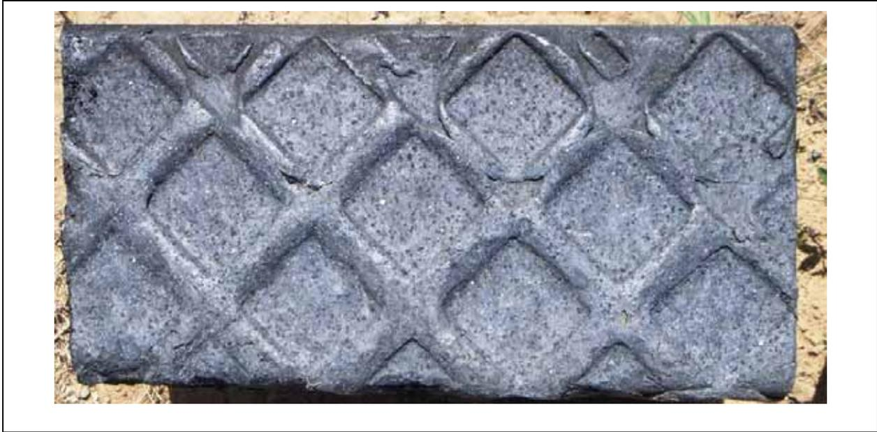
Figure 25. One of the plastic composite ties used for the electrical resistance laboratory test at TTCI.
