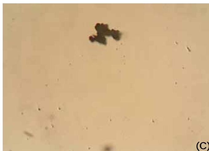
*Figure D6. Non-metallic inclusions in the different rail samples: (a) SW, (b) SU and (c) USA*
