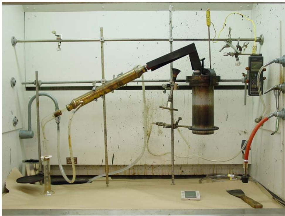
FIGURE 1 Picture of standard distillation method for emulsified asphalts.
