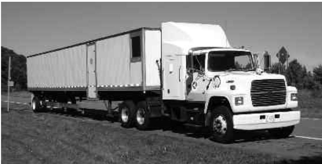
The rolling wheel deflectometer is a prototype device that measures pavement response to an actual moving wheel load.
