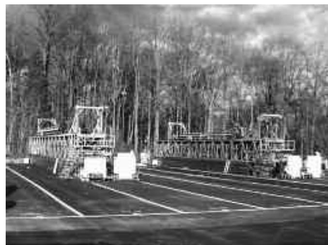
Accelerated pavement testing simulates the effects of long-term loading under in-service conditions.
