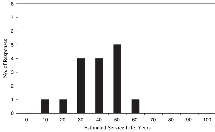
FIGURE 80 Estimated service life of corrugated metal drainage pipe.
