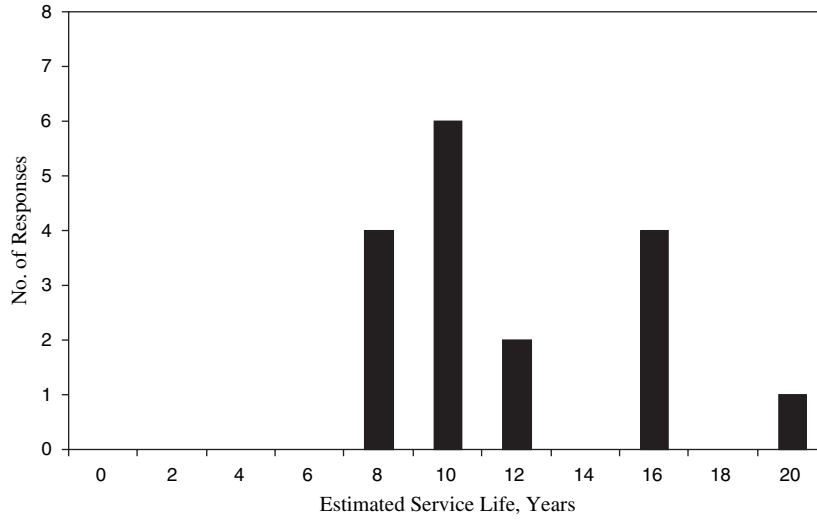
FIGURE 46 Estimated service life of sign sheeting undifferentiated by reflective performance or color.
