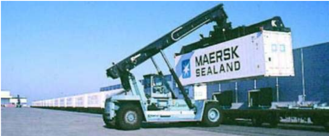
FIGURE 5 Top lifter used at APM Terminals, Port Elizabeth, New Jersey.
